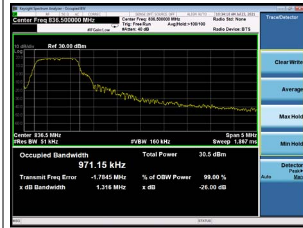
LTE eMTC Band 5 16QAM 5MHz CH-Middle
