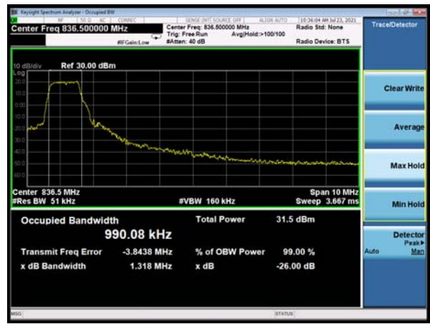
LTE eMTC Band 5 16QAM 10MHz CH-Middle
