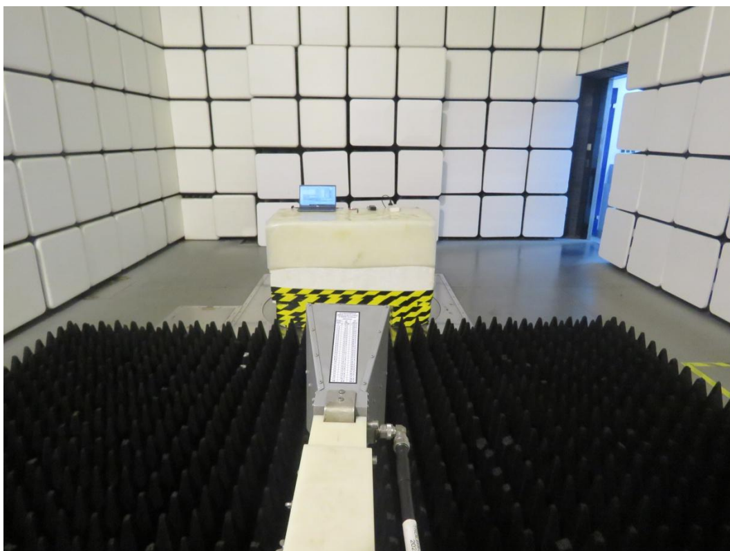
Picture 2: Receiver Spurious Emissions Test setup
