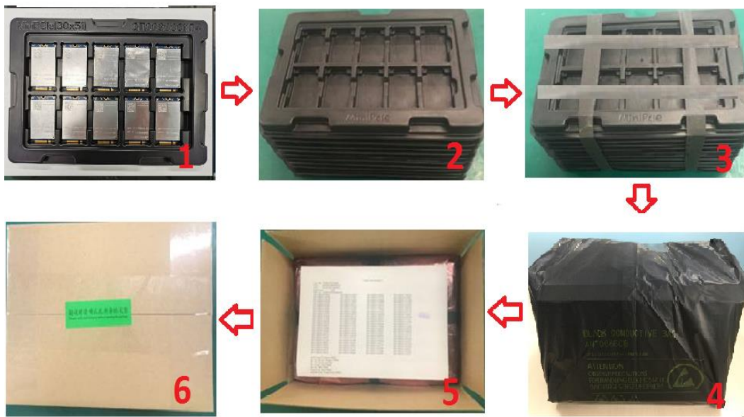
Figure 42: Tray Packaging Procedure
