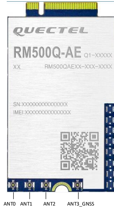
Figure 31: RM500Q-AE Antenna Connectors
