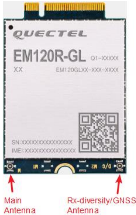
Figure 33: Antenna Connectors on the EM120R-GL Module
