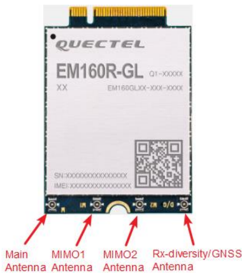
Figure 32: Antenna Connectors on the EM160R-GL Module
