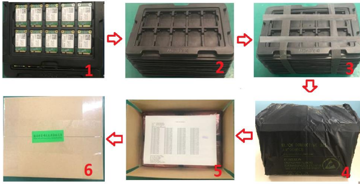
Figure 47: Tray Packaging Procedure
