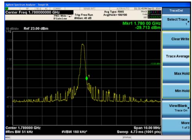
LTE Band 66 16QAM 1.4MHz CH-High, 100%
