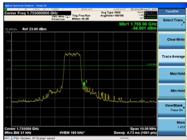
LTE Band 4 QPSK 5MHz CH-High, 100%RB
