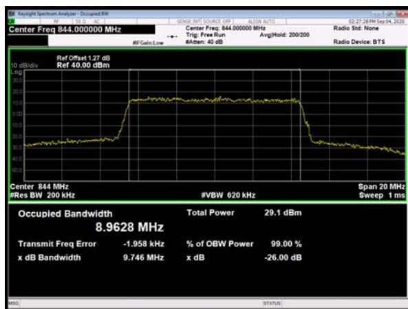
LTE Band 5 64QAM 10MHz CH-High
