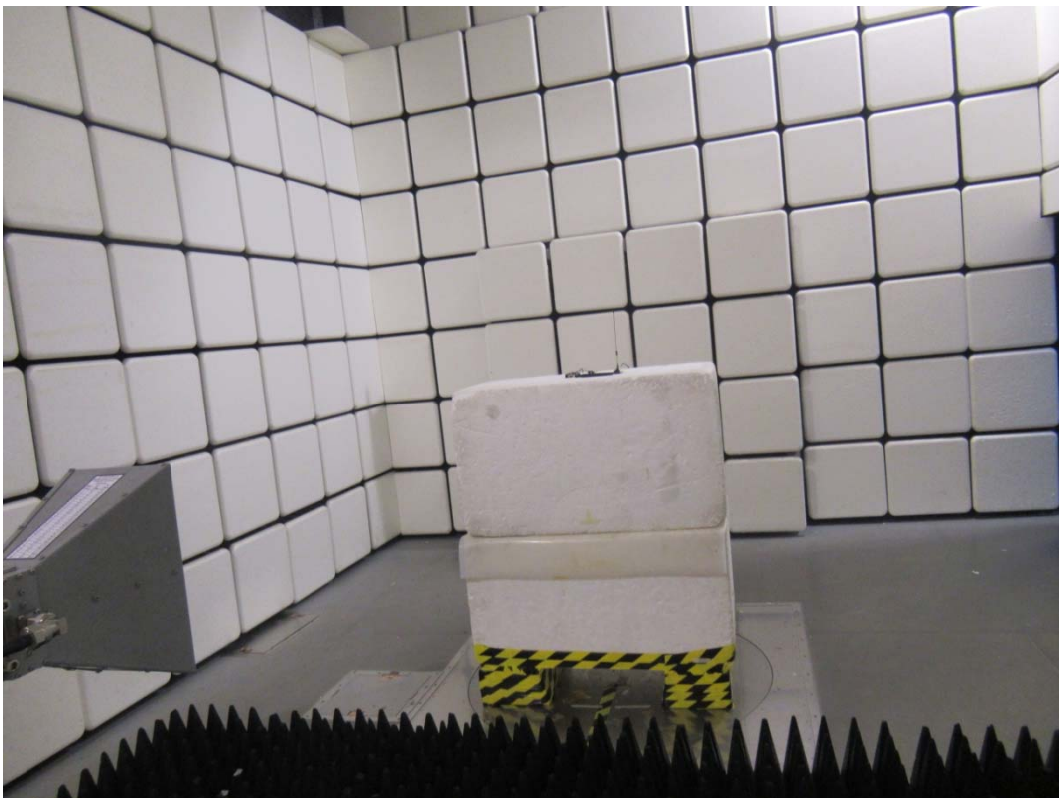
Picture 1: Radiated Spurious Emissions Test setup
