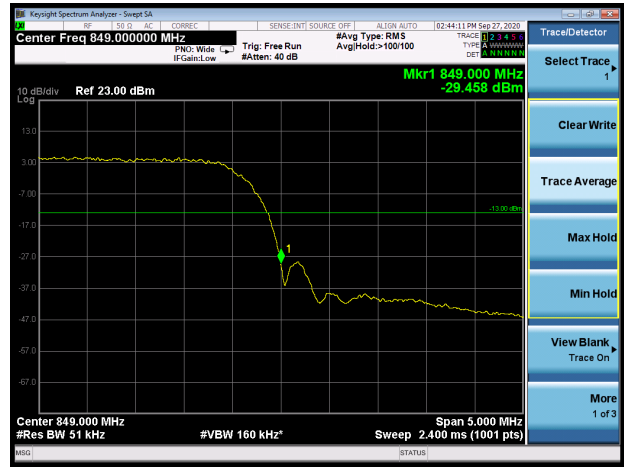
LTE Band 5 QPSK 1.4MHz CH-High 1RB
