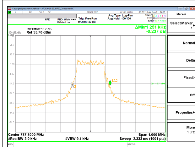
NB-IoT 15kHz High Channel subcarrier 12, carrier location 0
