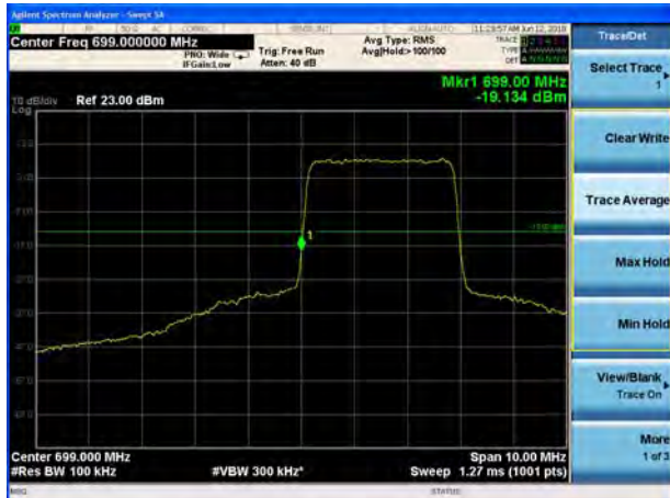
LTE Band 12 16QAM 5MHz CH-Low, 1 RB
