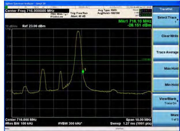
LTE Band 12 16QAM 3MHz CH-High, 100%RB
