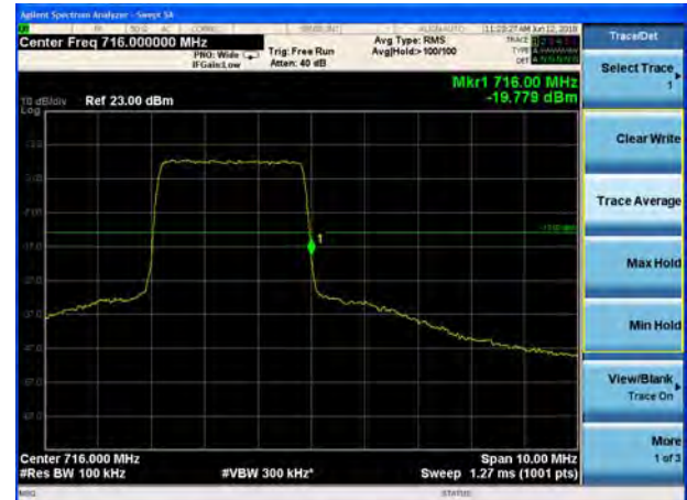
LTE Band 12 16QAM 5MHz CH-High, 1 RB
