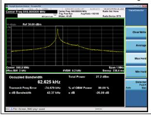
NB-IoT Band 5 QPSK 15kHz 1@0 CH-High
