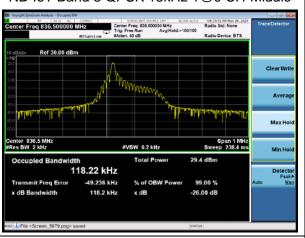
NB-IoT Band 5 QPSK 3.75kHz 1@0 CH-High
