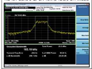
NB-IoT Band 5 QPSK 15kHz 12@0 CH-High
