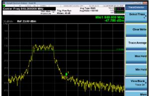
NB-IoT Band 5 QPSK 15kHz 12@0 CH-High
