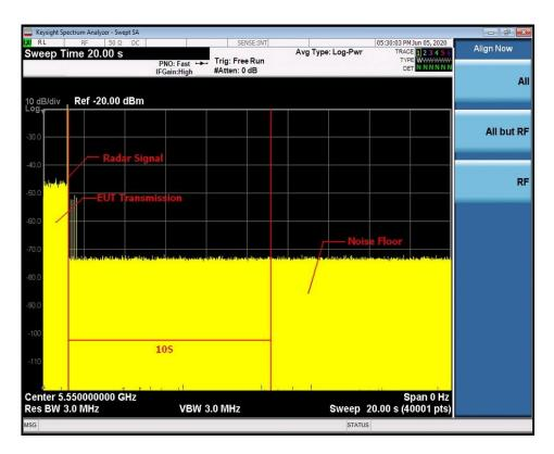
Note: An expanded plot for the device vacates the channel in the required 500ms
