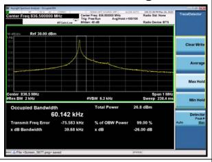
NB-IoT Band 5 QPSK 15kHz 1@0 CH-Middle
