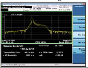
NB-IoT Band 5 QPSK 3.75kHz 1@0 CH-High
