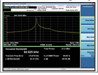
NB-IoT Band 5 QPSK 15kHz 1@0 CH-High
