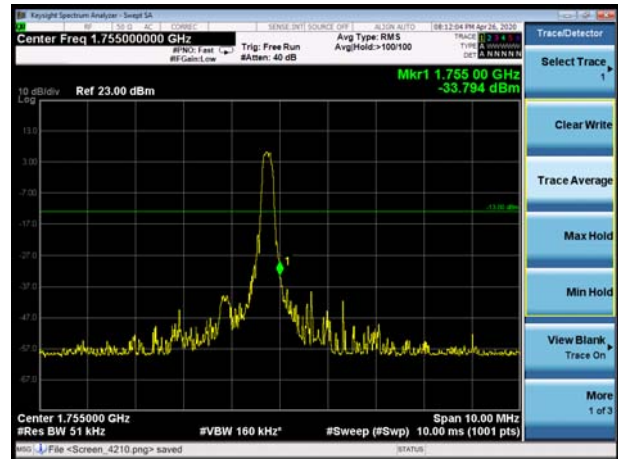
LTE Band 4 16QAM 1.4MHz CH-High, 100%RB
