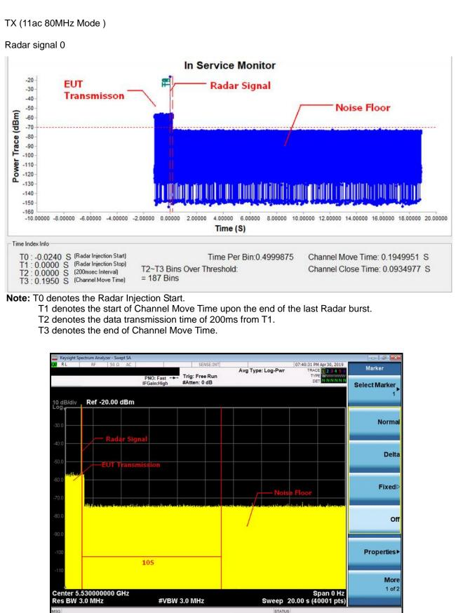
Note: An expanded plot for the device vacates the channel in the required 500ms
