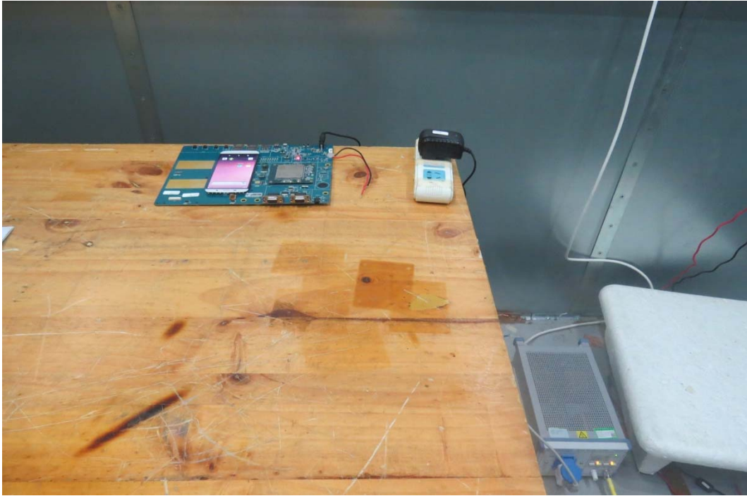
Picture 2 Conducted Emission Test Setup
