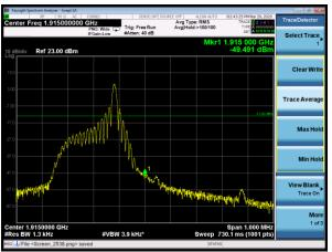
NB-IOT Band 25 QPSK 15kHz 12@0 CH-Low
