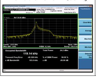
NB-IOT Band 25 QPSK 3.75kHz 1@0 CH-High
