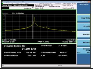
NB-IOT Band 2 QPSK 15kHz 12@0 CH-High
