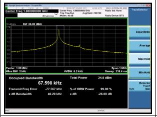
NB-IOT Band 2 QPSK 15kHz 1@0 CH-Middle
