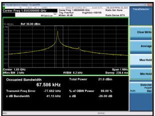
NB-IOT Band 25 BPSK 15kHz 1@0 CH-Middle
