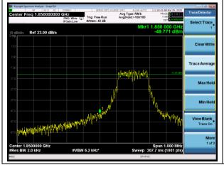
NB-IOT Band 2 QPSK 15kHz 12@0 CH-High
