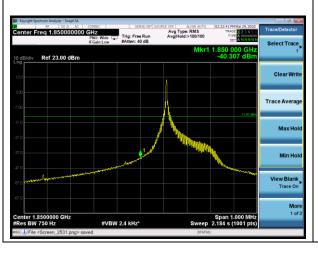
NB-IOT Band 25 QPSK 3.75kHz 1@47 CH-High
