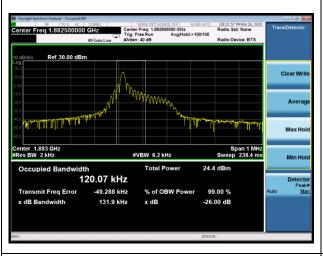
NB-IOT Band 25 QPSK 15kHz 12@0 CH-Middle
