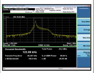
NB-IOT Band 25 QPSK 3.75kHz 1@0 CH-Middle
