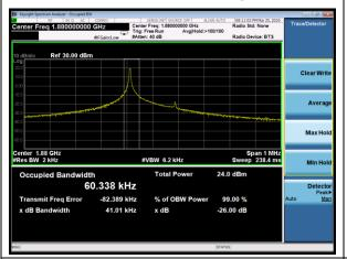
NB-IOT Band 2 BPSK 15kHz 1@0 CH-Middle
