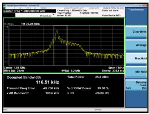
NB-IOT Band 2 QPSK 3.75kHz 1@0 CH-High
