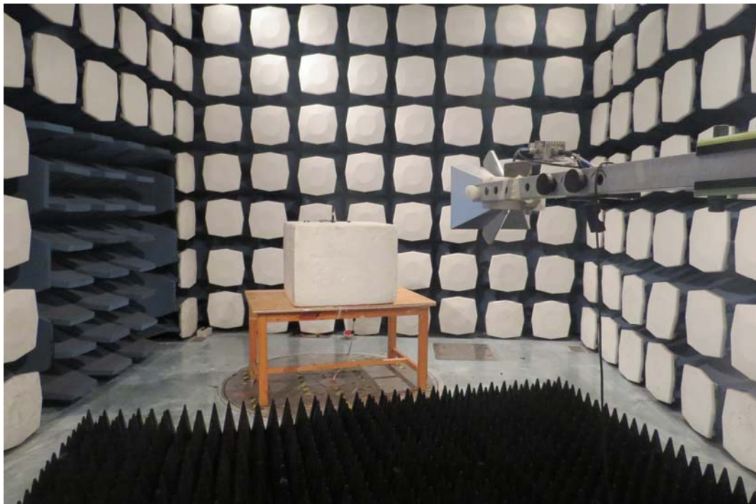
Picture 2: Radiated Spurious Emissions Test setup
