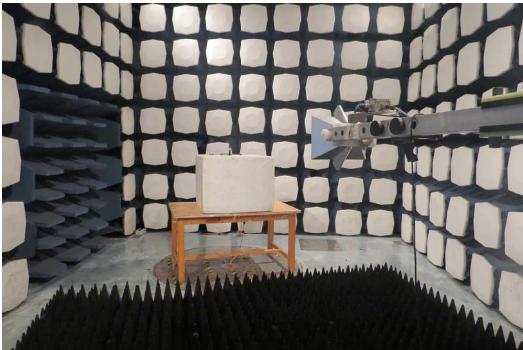
Picture 2: Radiated Spurious Emissions Test setup
