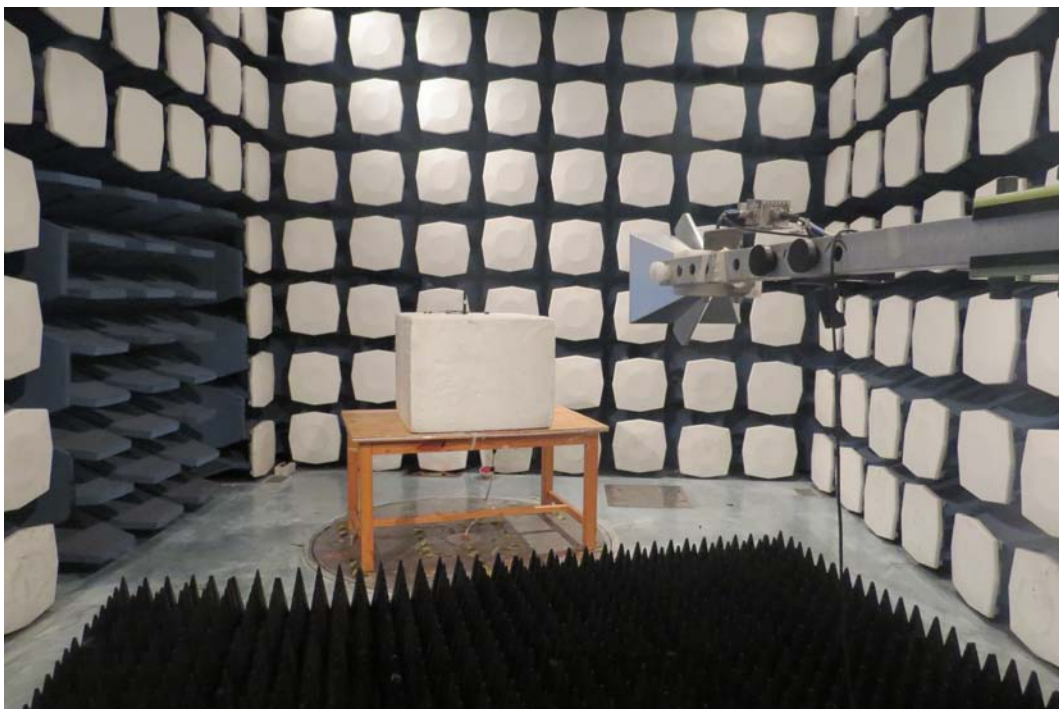
Picture 2: Radiated Spurious Emissions Test setup
