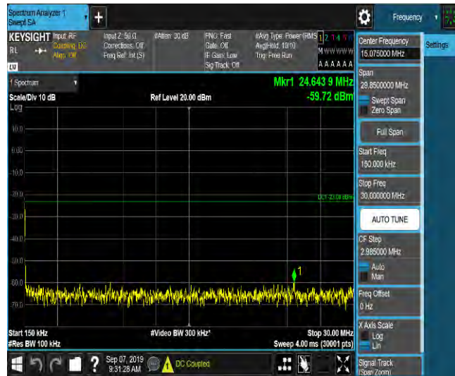
LTE Band 2_5MHz_QPSK_18900_1RB#0_Range3:30~1000MHz_-46.5_PASS
