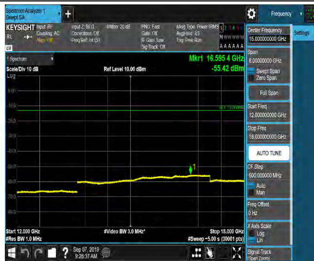
LTE Band 2_10MHz_16QAM_19150_1RB#0_Range1:0.009~0.15MHz_-63.4_PASS
