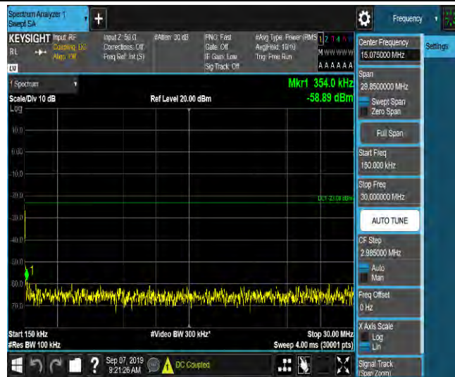
LTE Band 2_10MHz_QPSK_18900_1RB#0_Range3:30~1000MHz_-46.89_PASS
