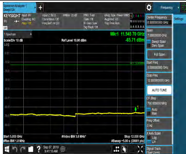
LTE Band 2_15MHz_16QAM_18675_1RB#0_Range6:12000~18000MHz_-55.46_PASS
