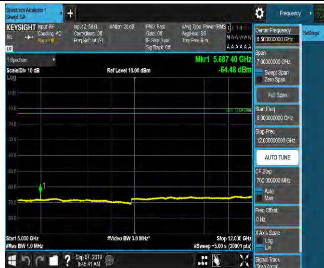
LTE Band 2_15MHz_QPSK_19125_1RB#0_Range6:12000~18000MHz_-55.39_PASS
