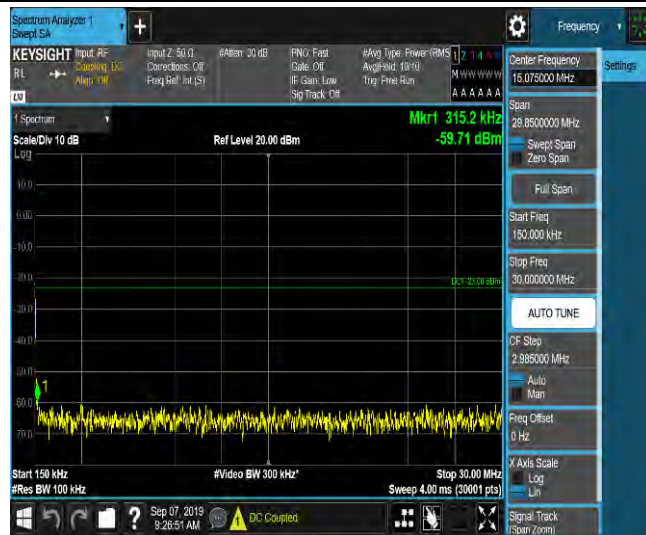
LTE Band 2_10MHz_16QAM_19150_1RB#0_Range3:30~1000MHz_-47_PASS
