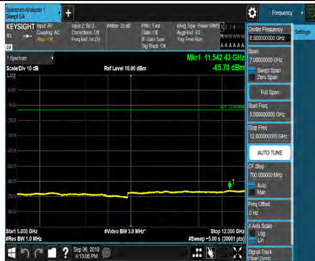
LTE Band 2_3MHz_16QAM_18615_1RB#0_Range6:12000~18000MHz_-55.32_PASS
