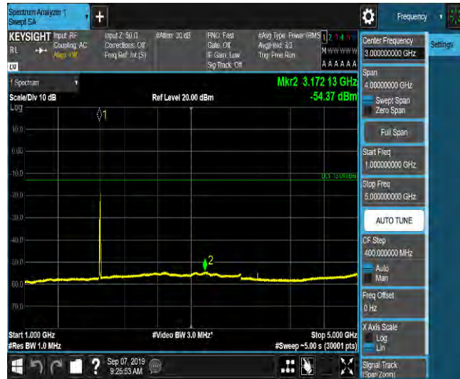
LTE Band 2_10MHz_QPSK_19150_1RB#0_Range5:5000~12000MHz_-64.39_PASS
