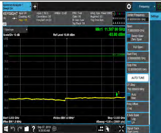
LTE Band 2_5MHz_16QAM_18900_1RB#0_Range6:12000~18000MHz_-55.48_PASS
