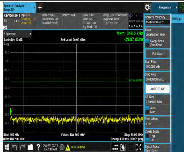
LTE Band 2_3MHz_QPSK_18900_1RB#0_Range3:30~1000MHz_-47.71_PASS
