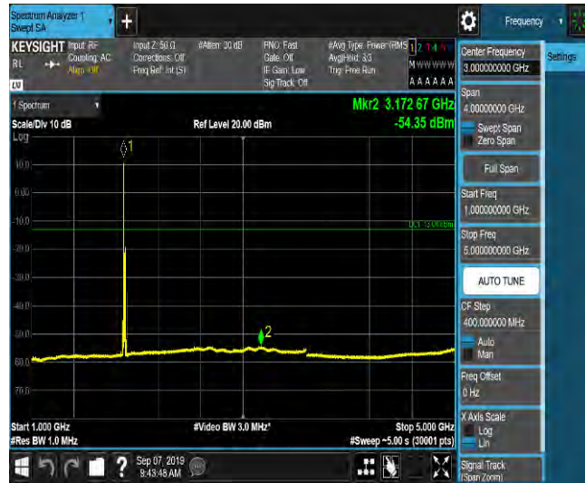
LTE Band 2_15MHz_16QAM_18900_1RB#0_Range5:5000~12000MHz_-65.75_PASS
