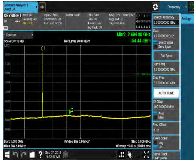
LTE Band 2_3MHz_16QAM_19185_1RB#0_Range5:5000~12000MHz_-63.72_PASS
