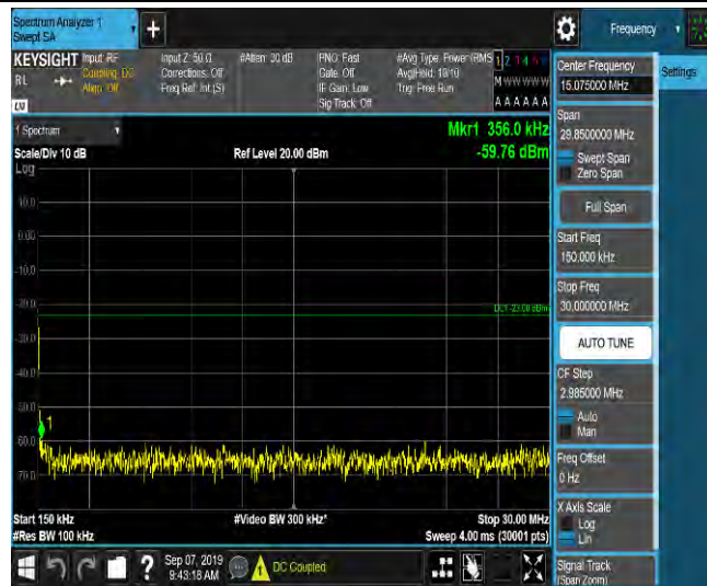
LTE Band 2_15MHz_16QAM_18900_1RB#0_Range3:30~1000MHz_-46.33_PASS
