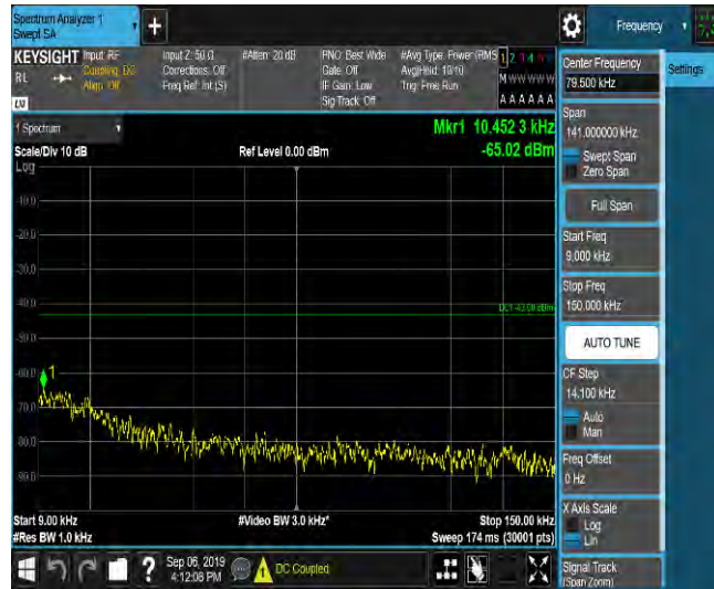
LTE Band 2_3MHz_16QAM_18615_1RB#0_Range2:0.15~30MHz_-59.5_PASS
