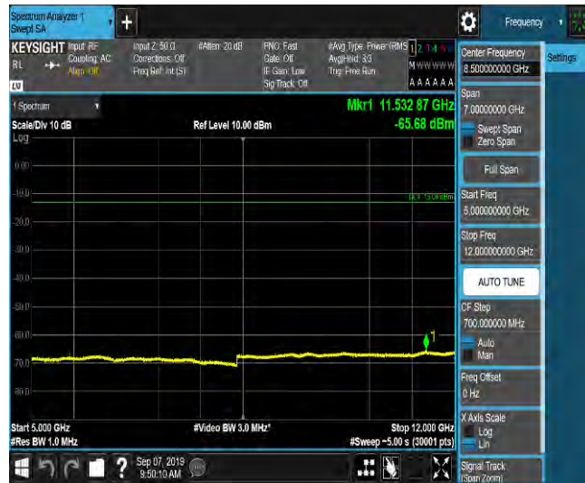
LTE Band 2_3MHz_16QAM_18900_1RB#0_Range6:12000~18000MHz_-55.31_PASS
