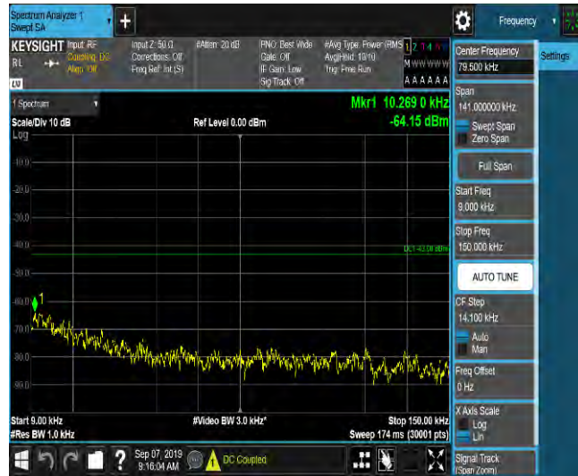
LTE Band 2_10MHz_QPSK_18650_1RB#0_Range2:0.15~30MHz_-59.87_PASS
