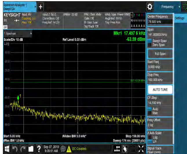
LTE Band 2_5MHz_16QAM_19175_1RB#0_Range2:0.15~30MHz_-58.65_PASS
