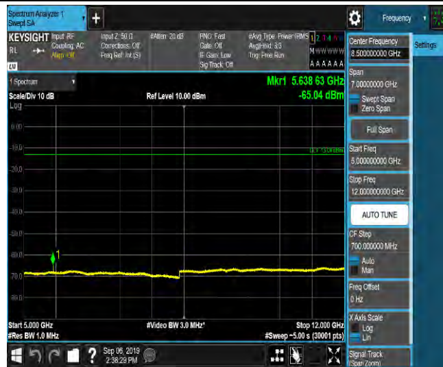
LTE Band 2_1.4MHz_QPSK_18900_1RB#0_Range6:12000~18000MHz_-55.35_PASS
