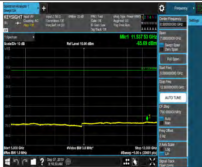
LTE Band 2_10MHz_16QAM_18650_1RB#0_Range6:12000~18000MHz_-55.47_PASS
