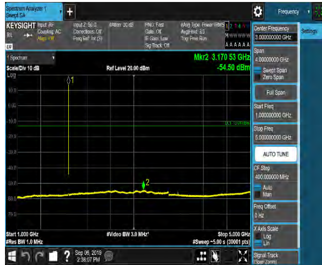
LTE Band 2_1.4MHz_QPSK_18900_1RB#0_Range5:5000~12000MHz_-65.05_PASS
