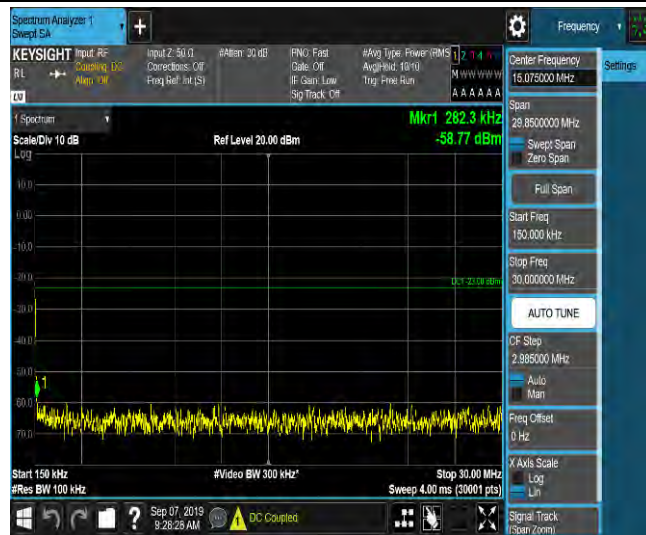
LTE Band 2_5MHz_QPSK_18625_1RB#0_Range3:30~1000MHz_-46.93_PASS
