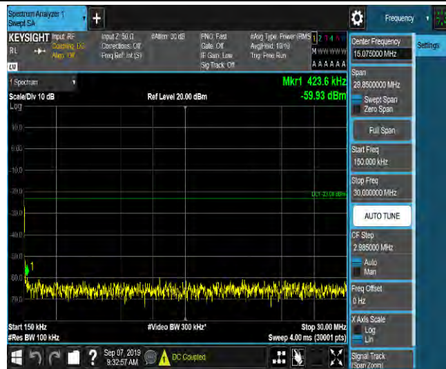
LTE Band 2_5MHz_16QAM_18900_1RB#0_Range3:30~1000MHz_-47.63_PASS
