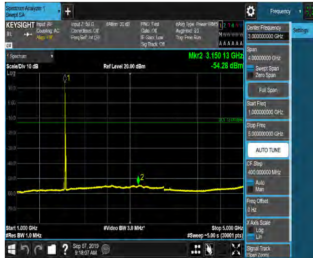
LTE Band 2_10MHz_16QAM_18650_1RB#0_Range5:5000~12000MHz_-65.69_PASS
