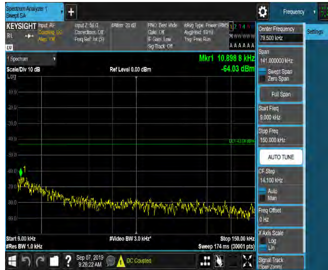
LTE Band 2_5MHz_QPSK_18625_1RB#0_Range2:0.15~30MHz_-58.77_PASS
