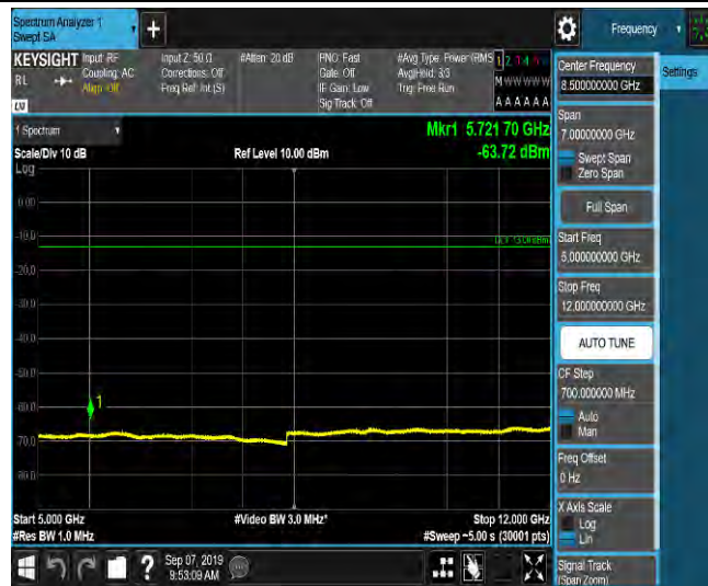
LTE Band 2_3MHz_16QAM_19185_1RB#0_Range6:12000~18000MHz_-55.47_PASS
