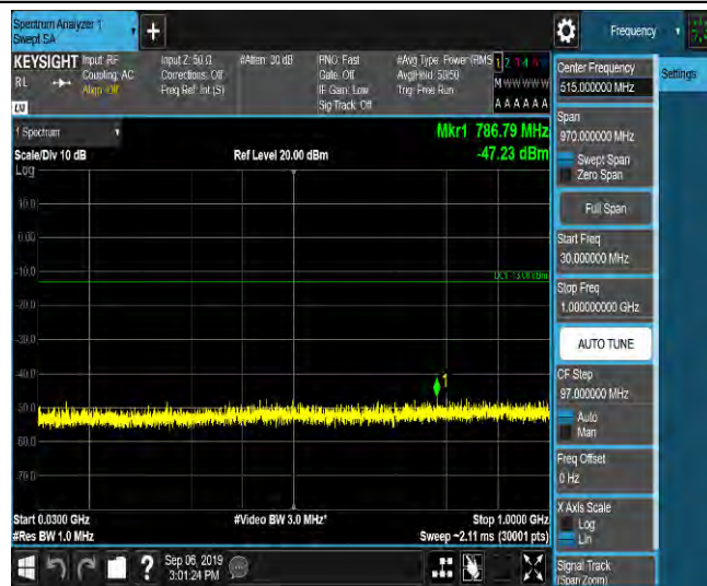
LTE Band 2_1.4MHz_16QAM_19193_1RB#0_Range4:1000~5000MHz_-54.29_PASS
