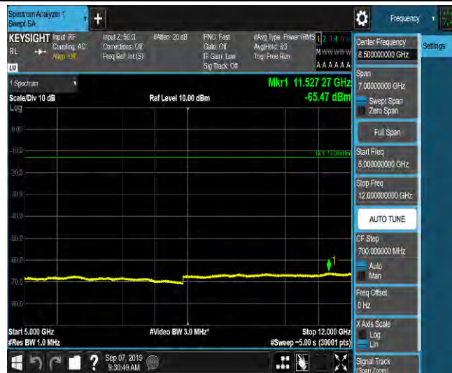
LTE Band 2_5MHz_16QAM_18625_1RB#0_Range6:12000~18000MHz_-55.5_PASS
