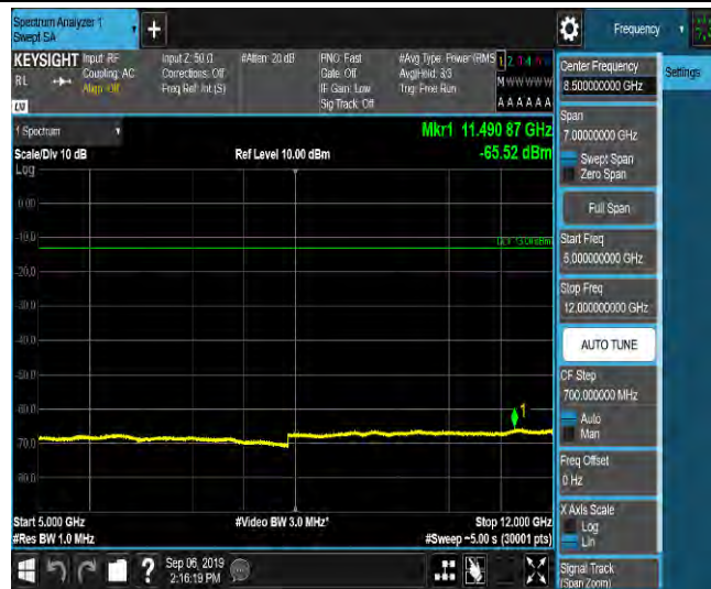
LTE Band 2_1.4MHz_QPSK_18607_1RB#0_Range6:12000~18000MHz_-55.35_PASS
