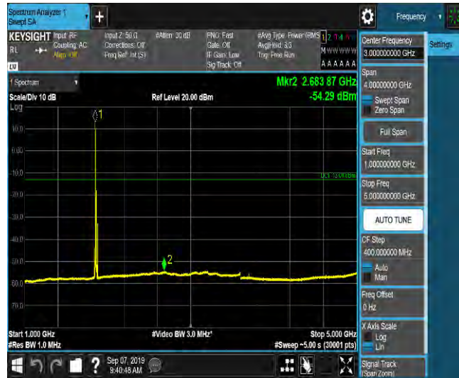
LTE Band 2_15MHz_16QAM_18675_1RB#0_Range5:5000~12000MHz_-65.71_PASS
