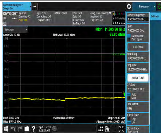
LTE Band 2_5MHz_QPSK_18625_1RB#0_Range6:12000~18000MHz_-55.42_PASS
