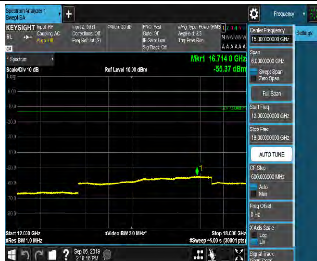
LTE Band 2_1.4MHz_QPSK_18900_1RB#0_Range1:0.009~0.15MHz_-62.68_PASS
