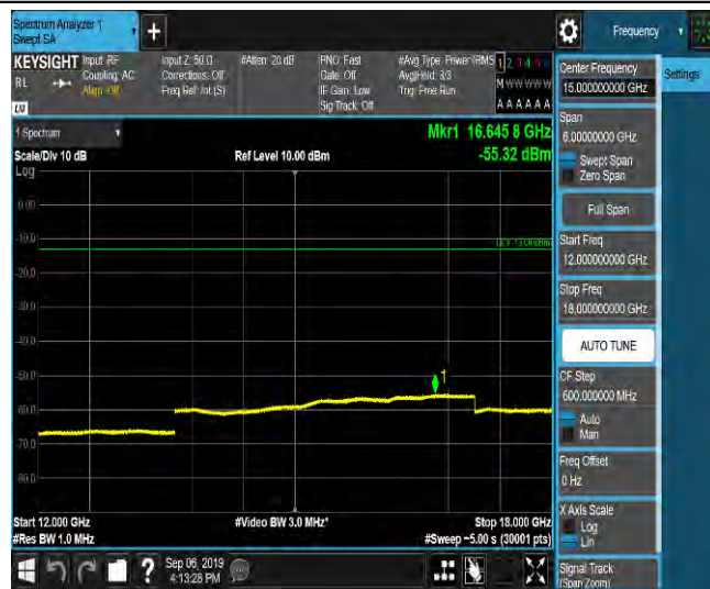
LTE Band 2_3MHz_QPSK_18900_1RB#0_Range1:0.009~0.15MHz_-63.48_PASS
