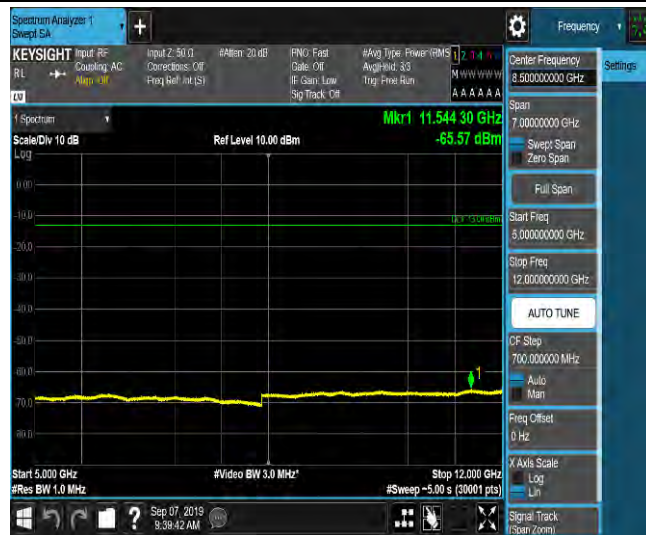
LTE Band 2_15MHz_QPSK_18675_1RB#0_Range6:12000~18000MHz_-55.5_PASS
