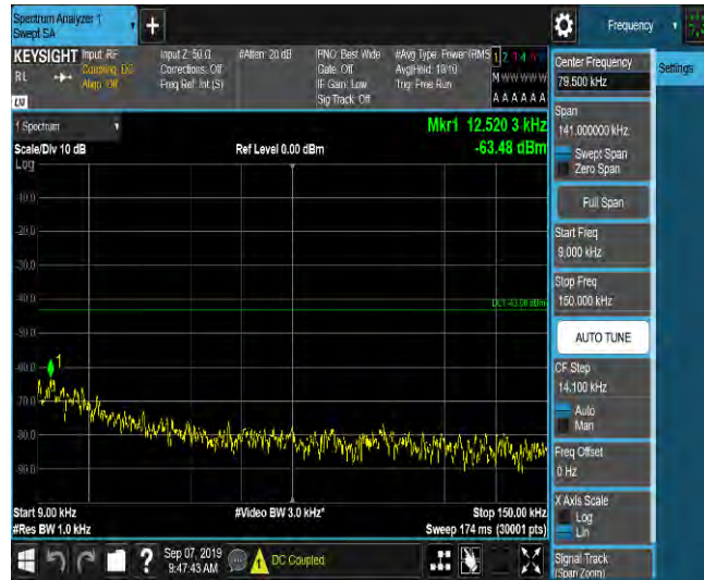
LTE Band 2_3MHz_QPSK_18900_1RB#0_Range2:0.15~30MHz_-59.97_PASS
