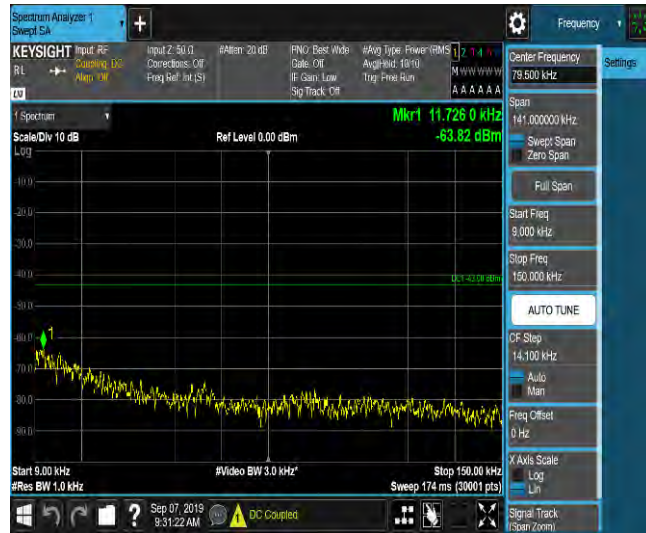
LTE Band 2_5MHz_QPSK_18900_1RB#0_Range2:0.15~30MHz_-59.72_PASS
