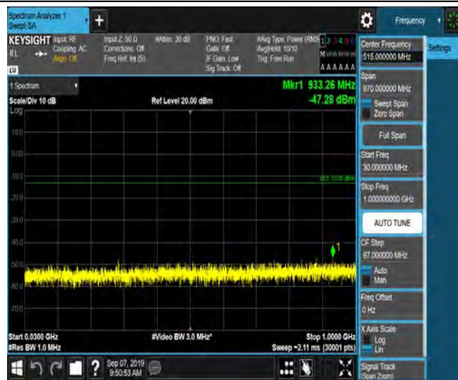
LTE Band 2_3MHz_QPSK_19185_1RB#0_Range4:1000~5000MHz_-54.43_PASS
