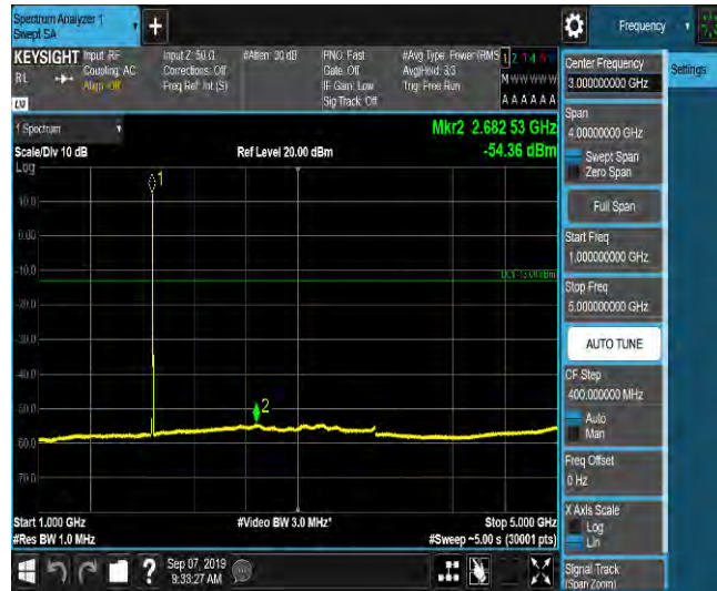
LTE Band 2_5MHz_16QAM_18900_1RB#0_Range5:5000~12000MHz_-65.8_PASS
