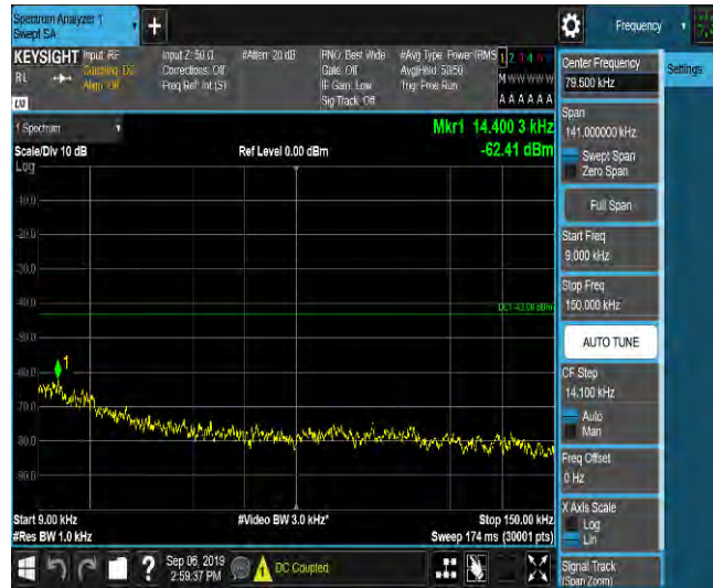
LTE Band 2_1.4MHz_QPSK_19193_1RB#0_Range2:0.15~30MHz_-57.76_PASS
