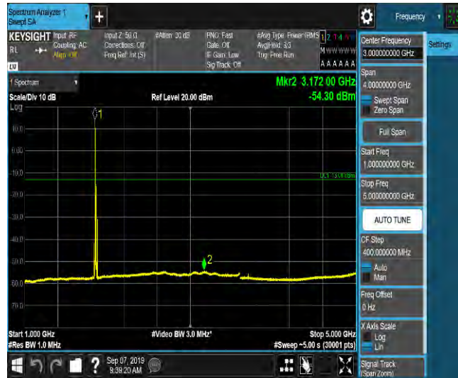
LTE Band 2_15MHz_QPSK_18675_1RB#0_Range5:5000~12000MHz_-65.57_PASS
