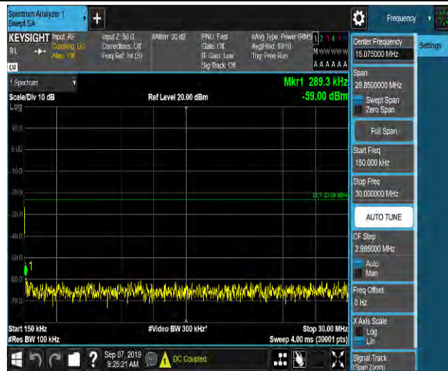
LTE Band 2_10MHz_QPSK_19150_1RB#0_Range3:30~1000MHz_-46.61_PASS
