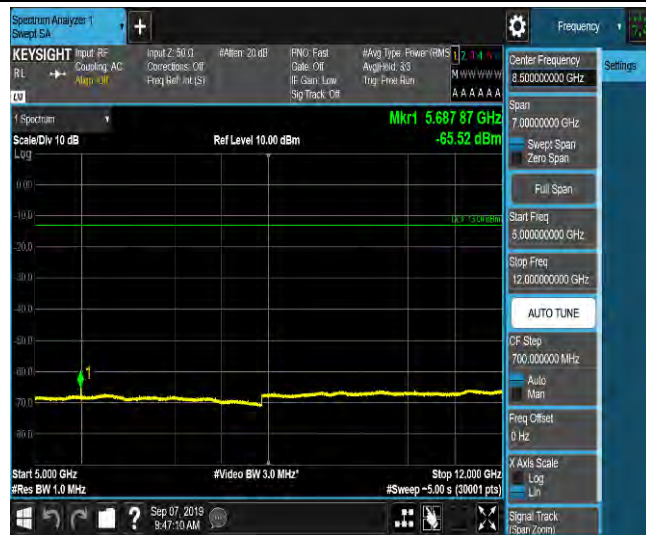
LTE Band 2_15MHz_16QAM_19125_1RB#0_Range6:12000~18000MHz_-55.45_PASS
