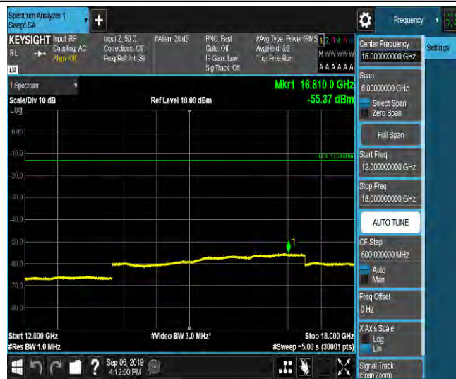
LTE Band 2_3MHz_16QAM_18615_1RB#0_Range1:0.009~0.15MHz_-65.02_PASS
