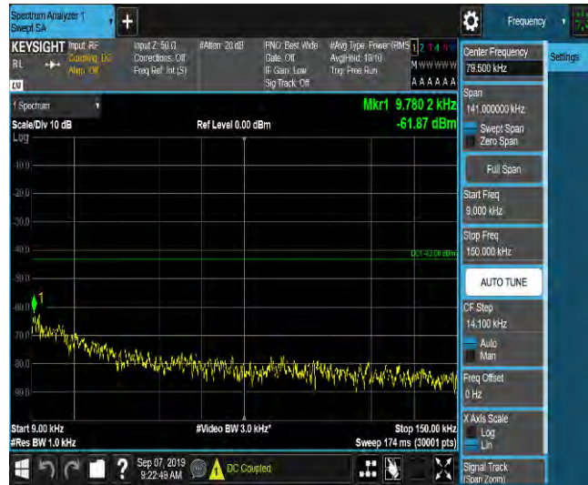
LTE Band 2_10MHz_16QAM_18900_1RB#0_Range2:0.15~30MHz_-60.78_PASS
