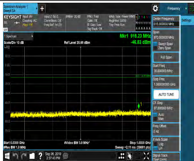
LTE Band 2_1.4MHz_QPSK_18900_1RB#0_Range4:1000~5000MHz_-54.5_PASS
