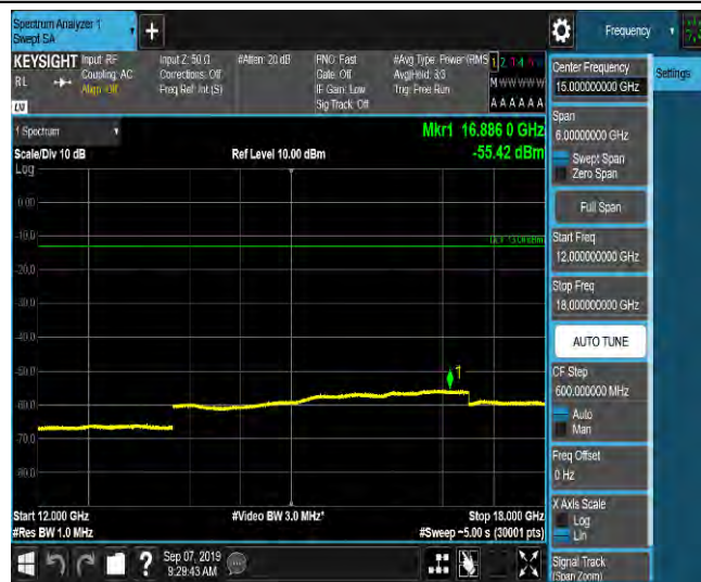
LTE Band 2_5MHz_16QAM_18625_1RB#0_Range1:0.009~0.15MHz_-62.97_PASS
