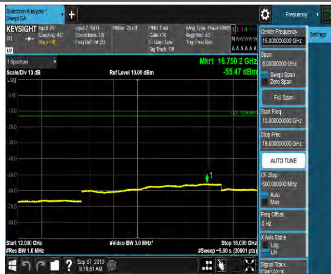
LTE Band 2_10MHz_QPSK_18900_1RB#0_Range1:0.009~0.15MHz_-63.76_PASS
