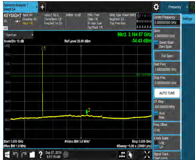
LTE Band 2_3MHz_QPSK_19185_1RB#0_Range5:5000~12000MHz_-63.08_PASS
