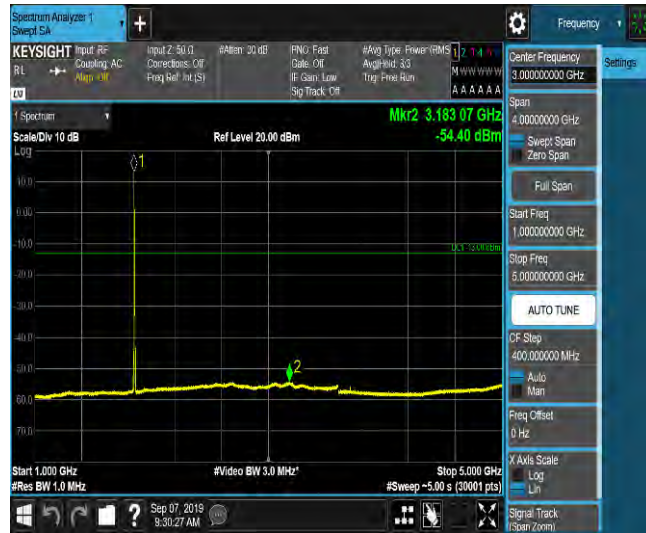
LTE Band 2_5MHz_16QAM_18625_1RB#0_Range5:5000~12000MHz_-65.47_PASS
