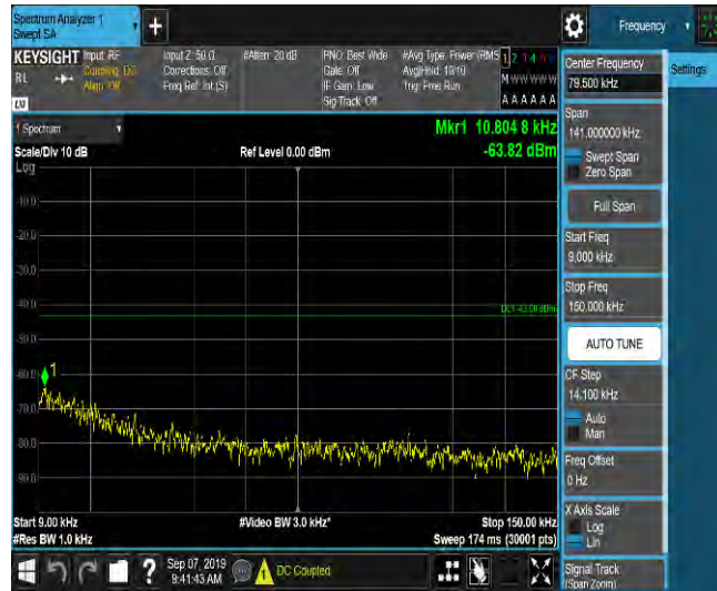
LTE Band 2_15MHz_QPSK_18900_1RB#0_Range2:0.15~30MHz_-59.24_PASS
