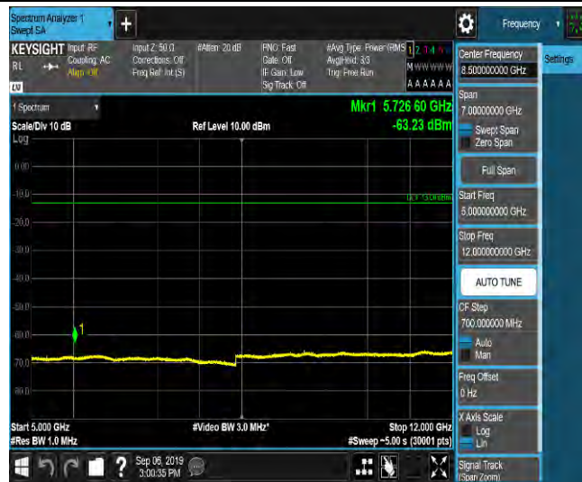
LTE Band 2_1.4MHz_QPSK_19193_1RB#0_Range6:12000~18000MHz_-55.34_PASS
