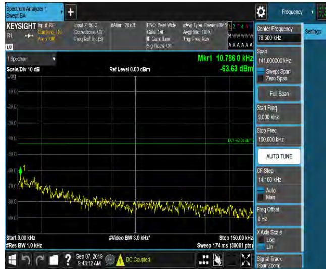
LTE Band 2_15MHz_16QAM_18900_1RB#0_Range2:0.15~30MHz_-59.76_PASS
