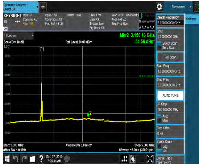
LTE Band 2_20MHz_QPSK_18700_1RB#0_Range5:5000~12000MHz_-65.56_PASS
