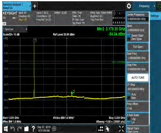
LTE Band 2_5MHz_QPSK_18900_1RB#0_Range5:5000~12000MHz_-65.57_PASS
