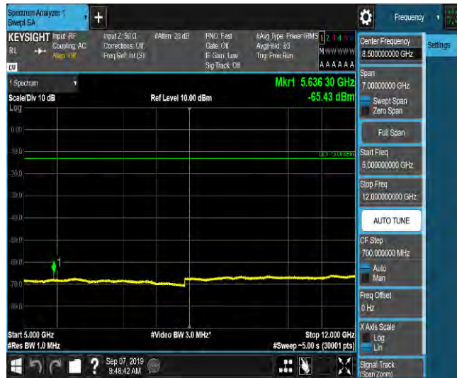
LTE Band 2_3MHz_QPSK_18900_1RB#0_Range6:12000~18000MHz_-55.38_PASS
