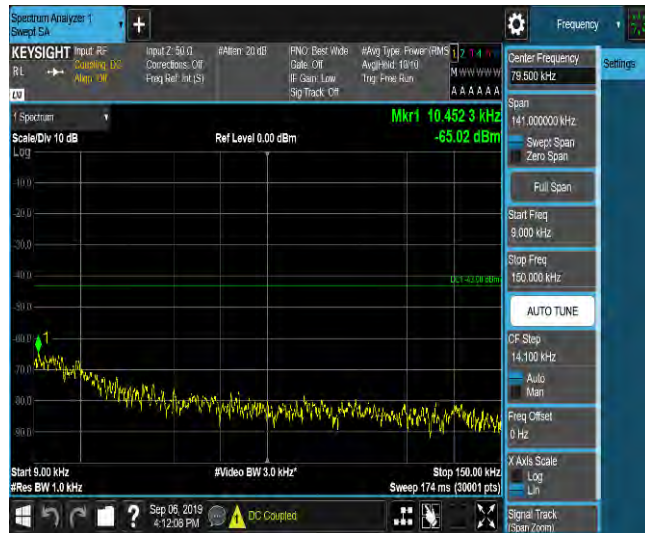
LTE Band 2_3MHz_16QAM_18615_1RB#0_Range2:0.15~30MHz_-59.5_PASS
