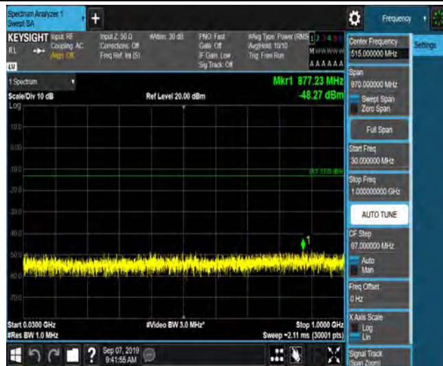
LTE Band 2_15MHz_QPSK_18900_1RB#0_Range4:1000~5000MHz_-54.38_PASS
