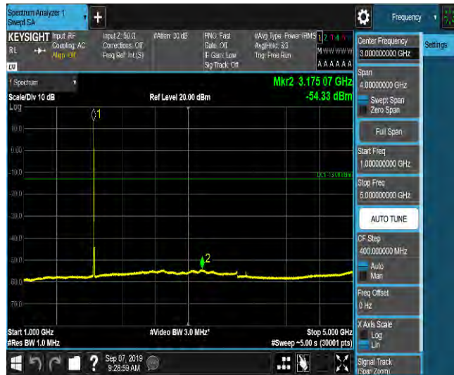
LTE Band 2_5MHz_QPSK_18625_1RB#0_Range5:5000~12000MHz_-65.85_PASS
