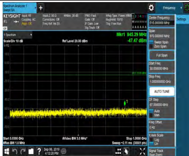
LTE Band 2_3MHz_16QAM_18615_1RB#0_Range4:1000~5000MHz_-54.41_PASS
