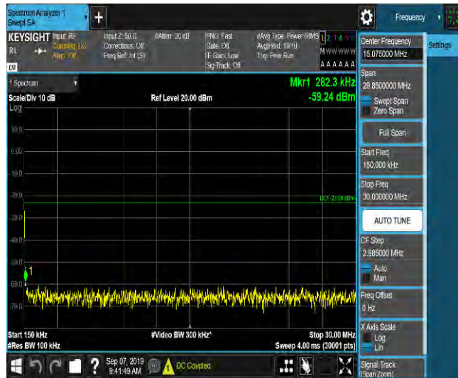
LTE Band 2_15MHz_QPSK_18900_1RB#0_Range3:30~1000MHz_-48.27_PASS
