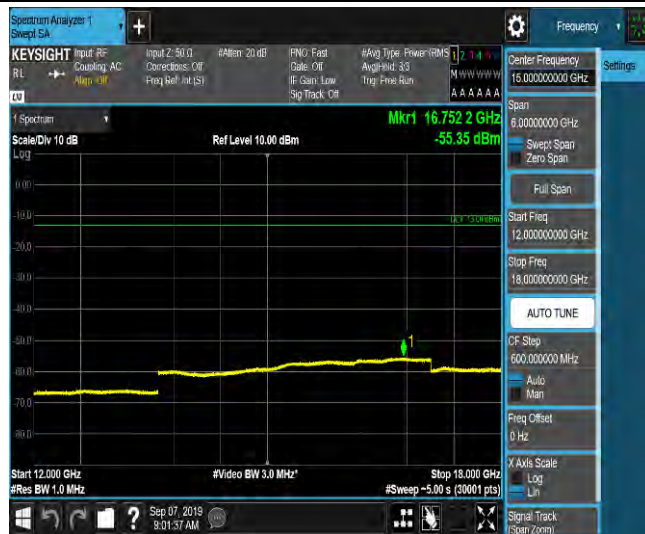
LTE Band 2_20MHz_16QAM_19100_1RB#0_Range1:0.009~0.15MHz_-63.8_PASS
