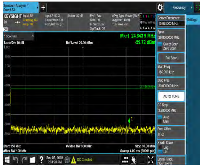
LTE Band 2_5MHz_QPSK_18900_1RB#0_Range3:30~1000MHz_-46.5_PASS
