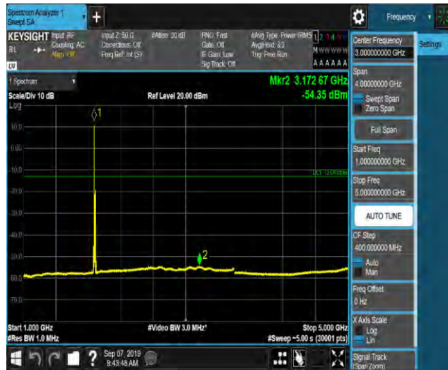
LTE Band 2_15MHz_16QAM_18900_1RB#0_Range5:5000~12000MHz_-65.75_PASS
