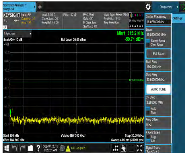
LTE Band 2_10MHz_16QAM_19150_1RB#0_Range3:30~100MHz_-47_PASS
