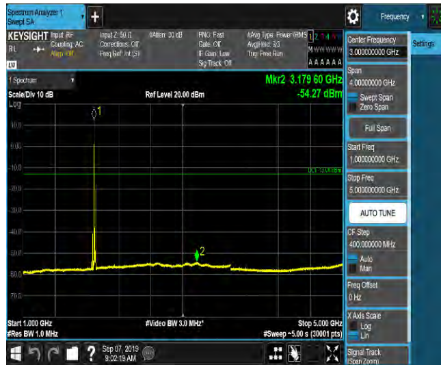
LTE Band 2_20MHz_16QAM_19100_1RB#0_Range5:5000~12000MHz_-65.09_PASS
