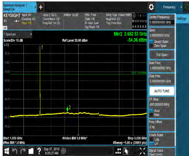
LTE Band 2_5MHz_16QAM_18900_1RB#0_Range5:5000~12000MHz_-65.8_PASS
