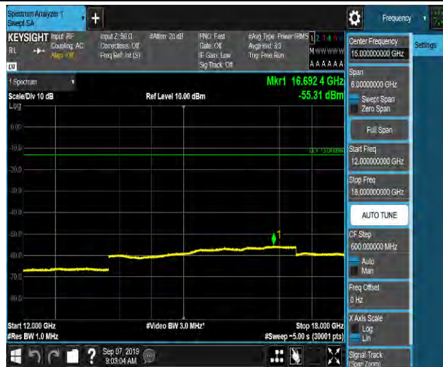
LTE Band 2_20MHz_16QAM_19100_1RB#0_Range6:12000~18000MHz_-55.31_PASS
