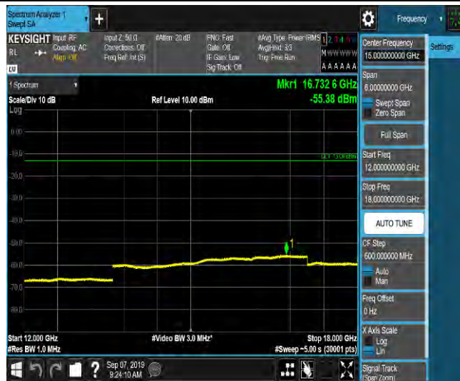
LTE Band 2_10MHz_QPSK_19150_1RB#0_Range1:0.009~0.15MHz_-64.96_PASS
