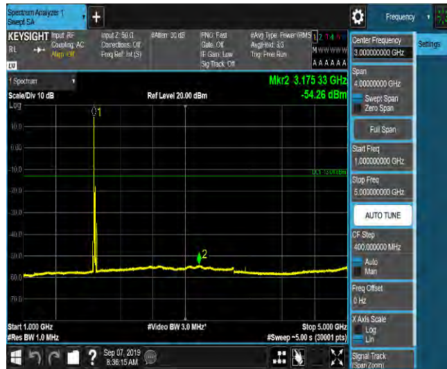
LTE Band 2_20MHz_QPSK_18900_1RB#0_Range5:5000~12000MHz_-65.76_PASS
