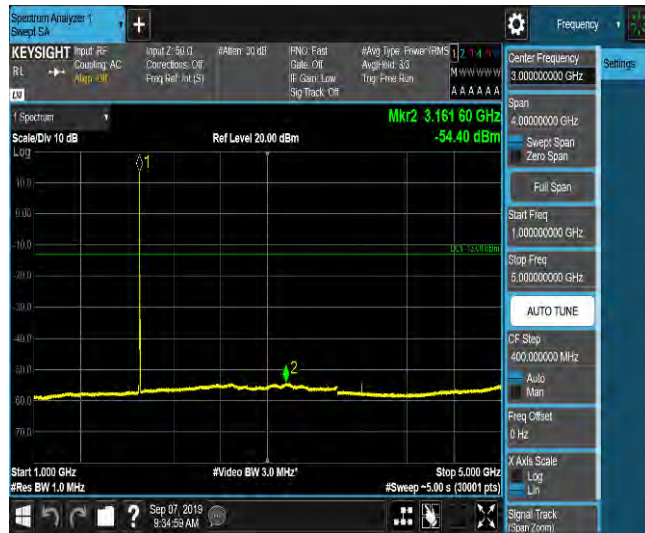
LTE Band 2_5MHz_QPSK_19175_1RB#0_Range5:5000~12000MHz_-63.86_PASS
