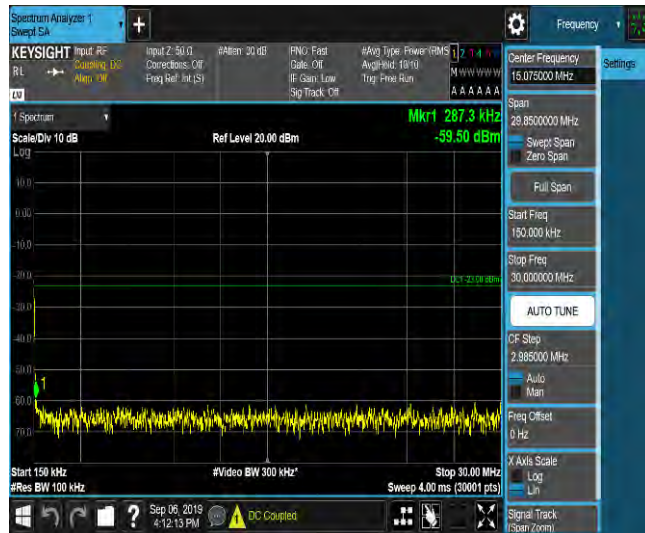
LTE Band 2_3MHz_16QAM_18615_1RB#0_Range3:30~1000MHz_-47.47_PASS
