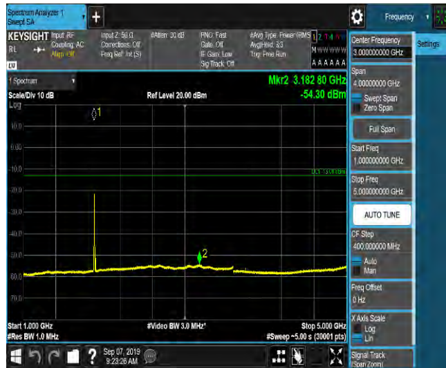
LTE Band 2_10MHz_16QAM_18900_1RB#0_Range5:5000~12000MHz_-65.69_PASS
