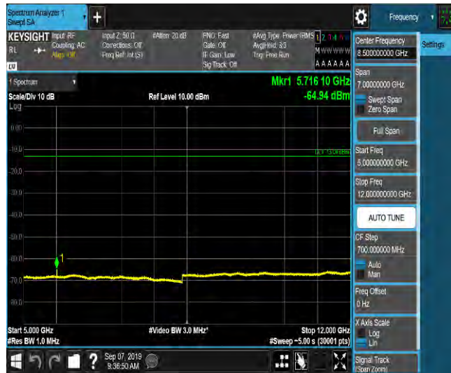
LTE Band 2_5MHz_16QAM_19175_1RB#0_Range6:12000~18000MHz_-55.45_PASS
