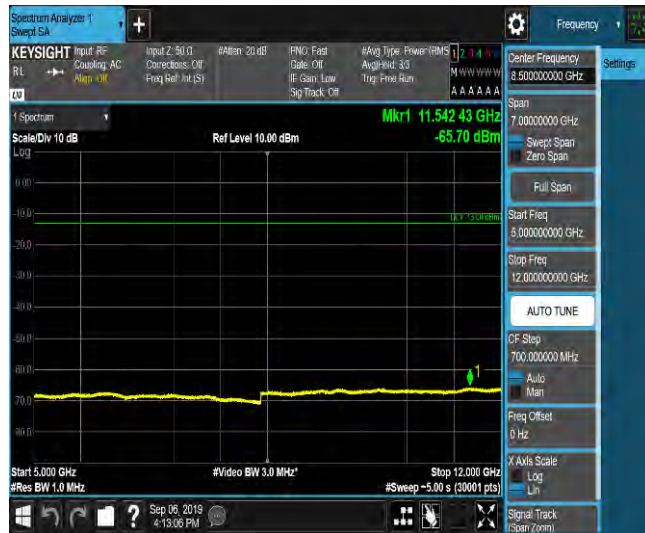
LTE Band 2_3MHz_16QAM_18615_1RB#0_Range6:12000~18000MHz_-55.32_PASS
