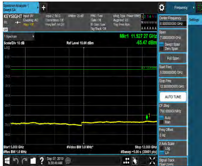
LTE Band 2_5MHz_16QAM_18625_1RB#0_Range6:12000~18000MHz_-55.5_PASS
