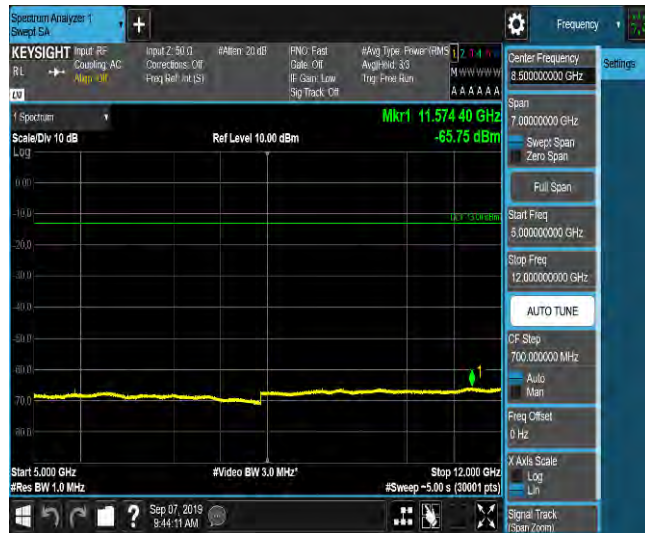
LTE Band 2_15MHz_16QAM_18900_1RB#0_Range6:12000~18000MHz_-55.52_PASS
