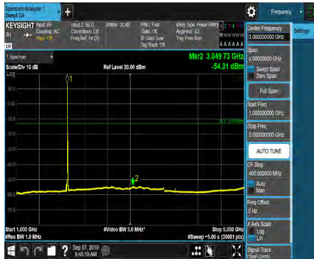
LTE Band 2_15MHz_QPSK_19125_1RB#0_Range5:5000~12000MHz_-64.48_PASS
