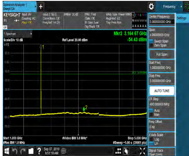
LTE Band 2_3MHz_QPSK_19185_1RB#0_Range5:5000~12000MHz_-63.08_PASS
