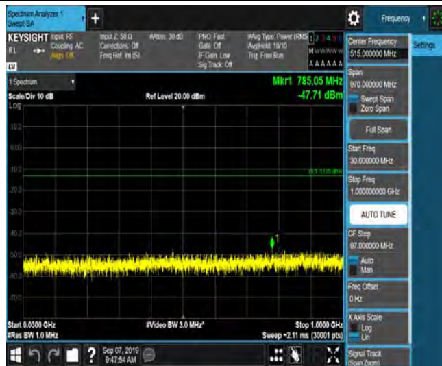
LTE Band 2_3MHz_QPSK_18900_1RB#0_Range4:1000~5000MHz_-54.29_PASS
