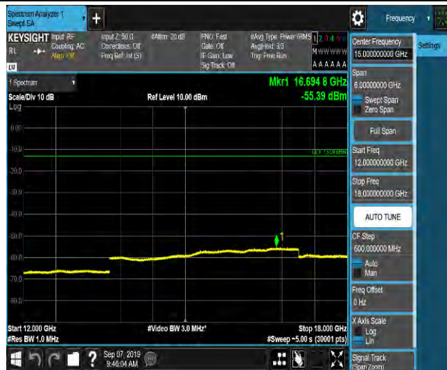
LTE Band 2_15MHz_16QAM_19125_1RB#0_Range1:0.009~0.15MHz_-63.08_PASS
