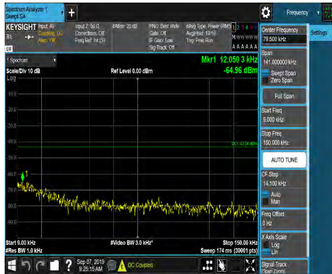
LTE Band 2_10MHz_QPSK_19150_1RB#0_Range2:0.15~30MHz_-59_PASS
