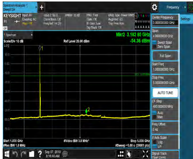
LTE Band 2_10MHz_QPSK_18650_1RB#0_Range5:5000~12000MHz_-65.7_PASS
