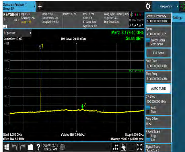
LTE Band 2_5MHz_16QAM_19175_1RB#0_Range5:5000~12000MHz_-64.94_PASS
