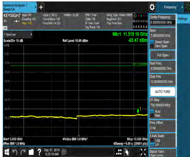
LTE Band 2_10MHz_QPSK_18900_1RB#0_Range6:12000~18000MHz_-55.38_PASS
