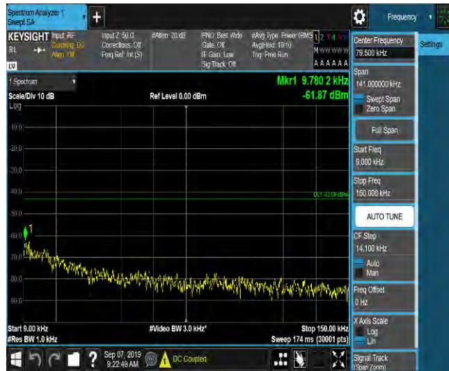
LTE Band 2_10MHz_16QAM_18900_1RB#0_Range2:0.15~30MHz_-60.78_PASS
