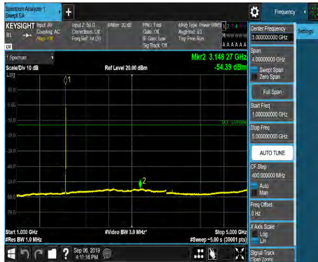
LTE Band 2_3MHz_QPSK_18615_1RB#0_Range5:5000~12000MHz_-65.64_PASS
