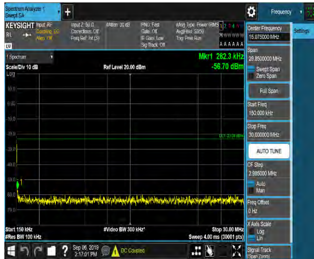
LTE Band 2_1.4MHz_16QAM_18607_1RB#0_Range3:30~1000MHz_-46.58_PASS
