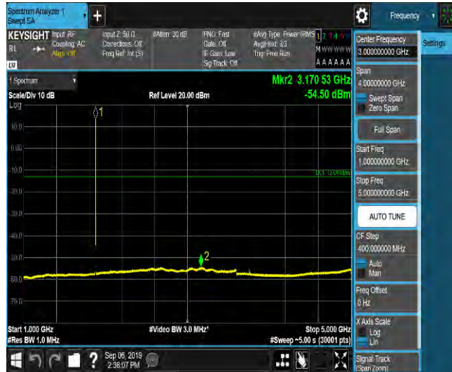
LTE Band 2_1.4MHz_QPSK_18900_1RB#0_Range5:5000~12000MHz_-65.05_PASS
