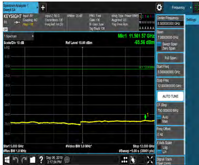
LTE Band 2_1.4MHz_16QAM_18607_1RB#0_Range6:12000~18000MHz_-55.37_PASS
