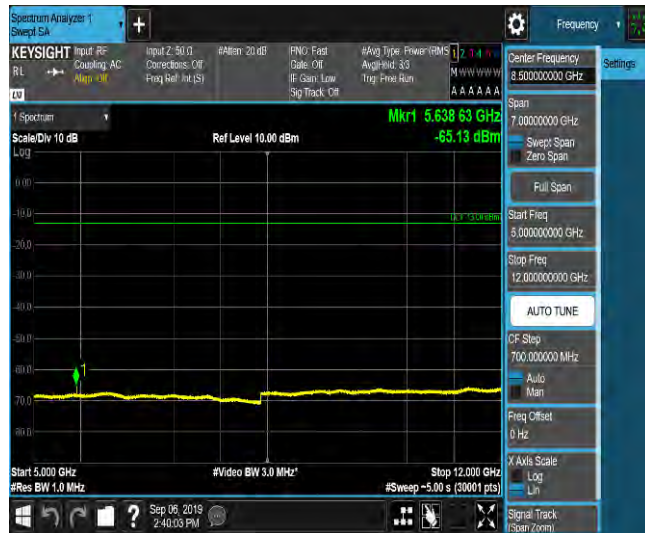
LTE Band 2_1.4MHz_16QAM_18900_1RB#0_Range6:12000~18000MHz_-55.17_PASS
