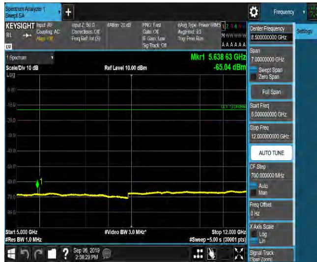
LTE Band 2_1.4MHz_QPSK_18900_1RB#0_Range6:12000~18000MHz_-55.35_PASS
