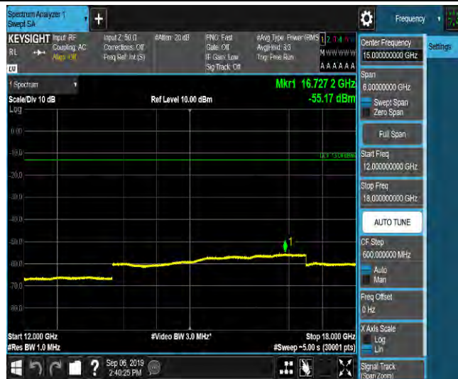
LTE Band 2_1.4MHz_QPSK_19193_1RB#0_Range1:0.009~0.15MHz_-62.41_PASS
