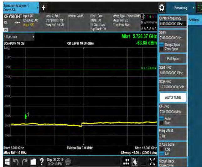
LTE Band 2_1.4MHz_16QAM_19193_1RB#0_Range6:12000~18000MHz_-55.28_PASS
