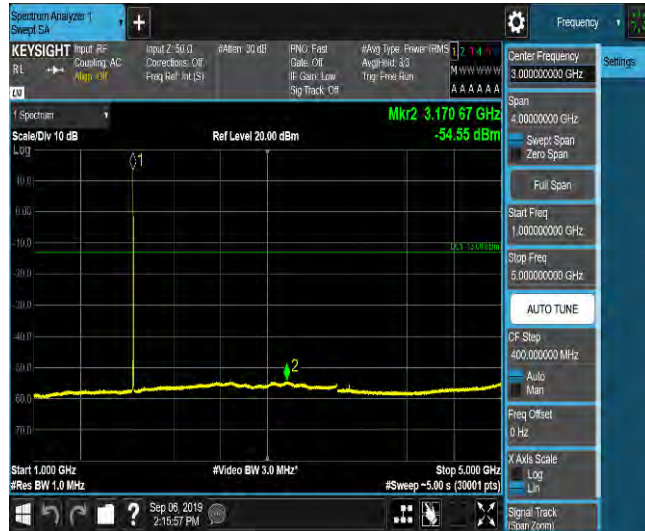
LTE Band 2_1.4MHz_QPSK_18607_1RB#0_Range5:5000~12000MHz_-65.52_PASS
