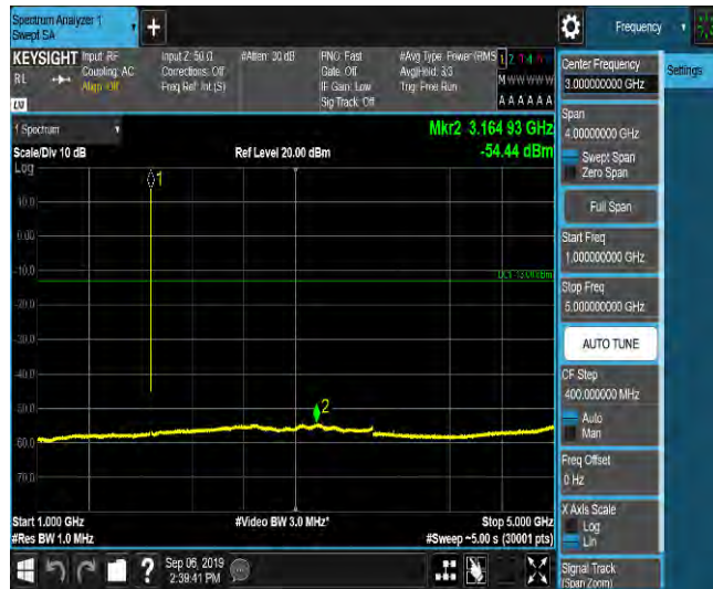
LTE Band 2_1.4MHz_16QAM_18900_1RB#0_Range5:5000~12000MHz_-65.13_PASS
