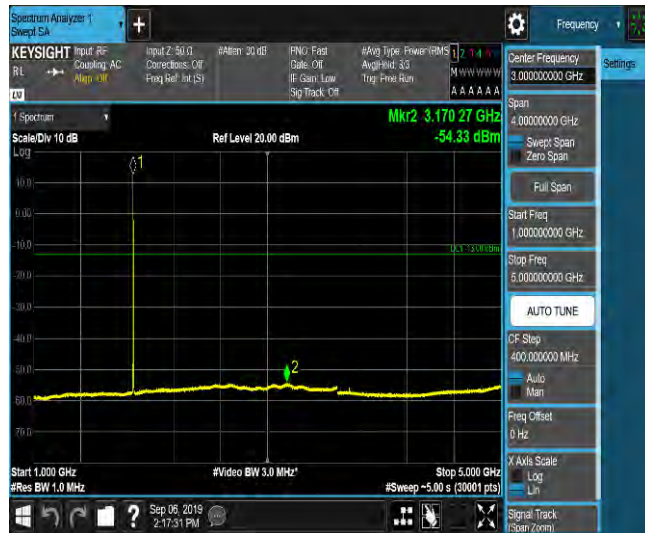
LTE Band 2_1.4MHz_16QAM_18607_1RB#0_Range5:5000~12000MHz_-65.56_PASS
