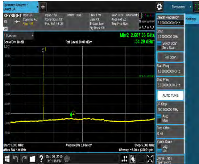
LTE Band 2_1.4MHz_16QAM_19193_1RB#0_Range5:5000~12000MHz_-63.85_PASS
