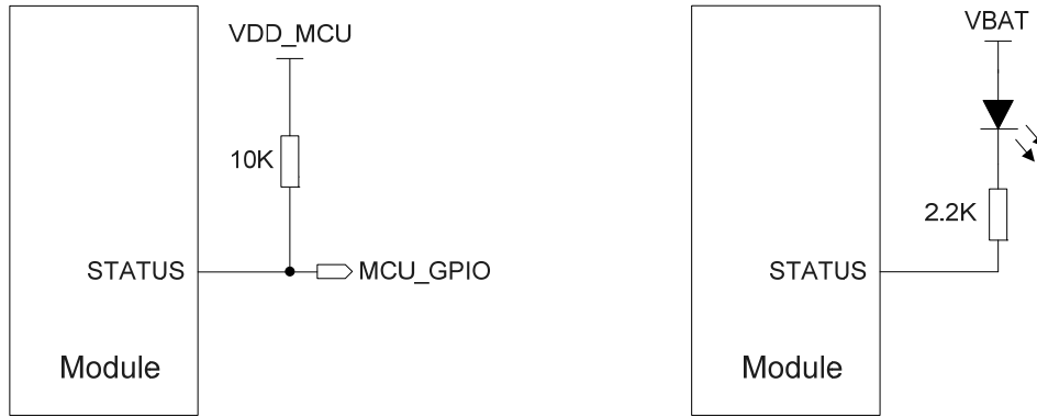
Figure 30: Reference Circuits of STATUS
