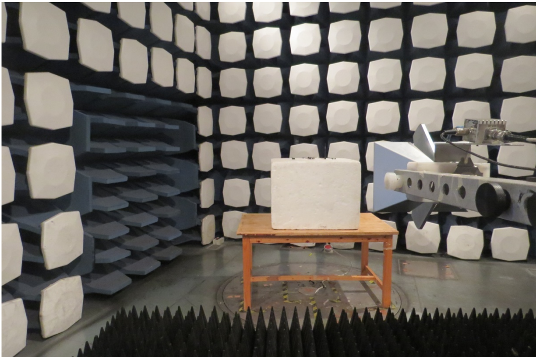
Radiated Spurious Emissions Test setup
