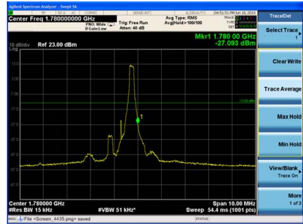
LTE Band 66 16QAM 1.4MHz CH-High, 100%RB
