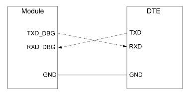
Figure 17: Reference Design of Debug UART Port
