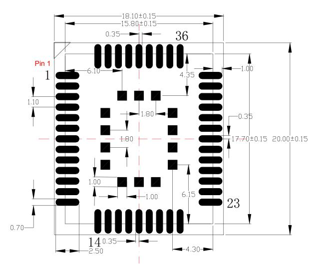
Figure 33: Recommended Footprint (Unit: mm)
