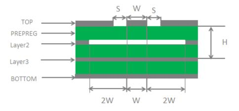
Figure 28: Coplanar Waveguide Line Design on a 4-layer PCB (Layer 3 as Reference Ground)
