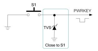
Figure 8: Turn on the Module Using Keystroke
