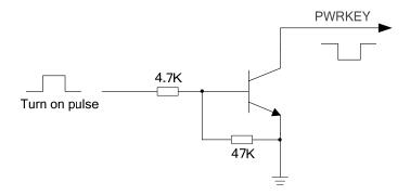
Figure 7: Turn on the Module Using Driving Circuit
