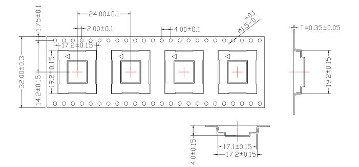
Figure 35: Tape Dimensions (Unit: mm)
