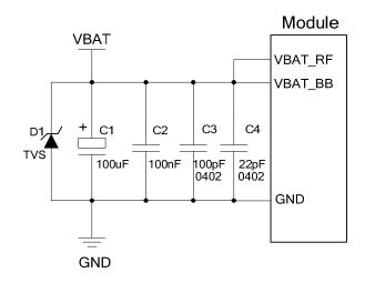
Figure 6: Reference Circuit for Power Supply
