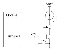
Figure 24: Reference Design of NETLIGHT
