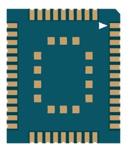
Figure 34: Bottom View of the Module
