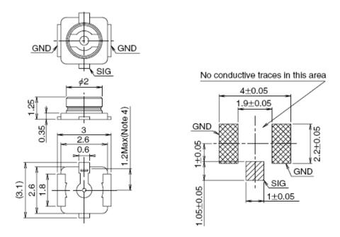
Figure 30: Dimensions of the U.FL-R-SMT Connector (Unit: mm)
