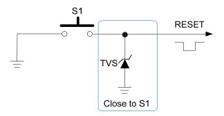
Figure 13: Reference Circuit of RESET by Using Button
