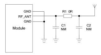
Figure 25: Reference Design of NB-IoT Antenna Interface
