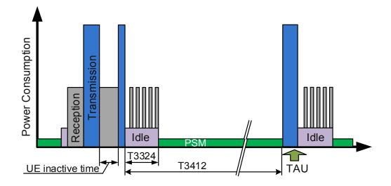
Figure 4: Module Power Consumption in Different Modes
