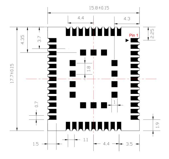
Figure 32: Module Bottom Dimension (Bottom View)
