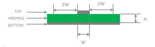
Figure 26: Microstrip Line Design on a 2-layer PCB
