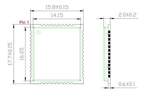
Figure 31: BC66-NA Top and Side Dimensions (Unit: mm)
