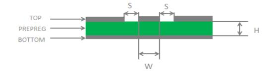
Figure 27: Coplanar Waveguide Line Design on a 2-layer PCB
