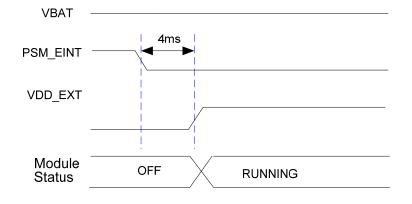
Figure 5: Timing of Waking up Module from PSM
