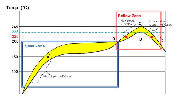
Figure 36: Recommended Reflow Soldering Thermal Profile
