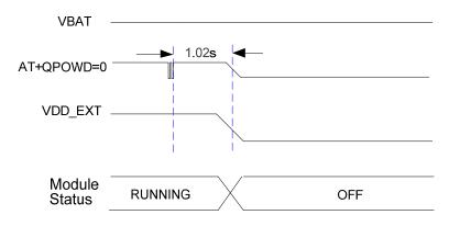
Figure 10: Power down Timing (Power off by AT Command)
