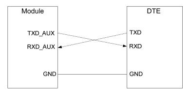
Figure 18: Reference Design of Auxiliary UART Port
