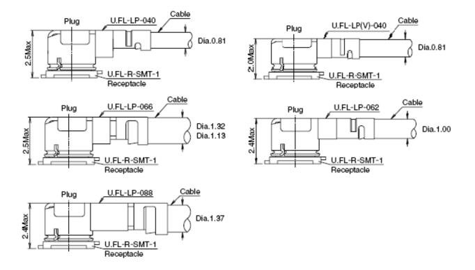
Figure 32: Space Factor of Mated Connector (Unit: mm)
