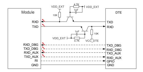
Figure 20: Reference Circuit with Transistor Circuit
