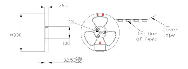
Figure 36: Reel Dimensions (Unit: mm)
