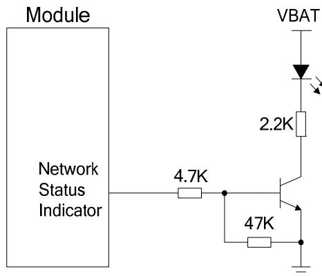
Figure 33: Reference Circuit of the Network Status Indicator
