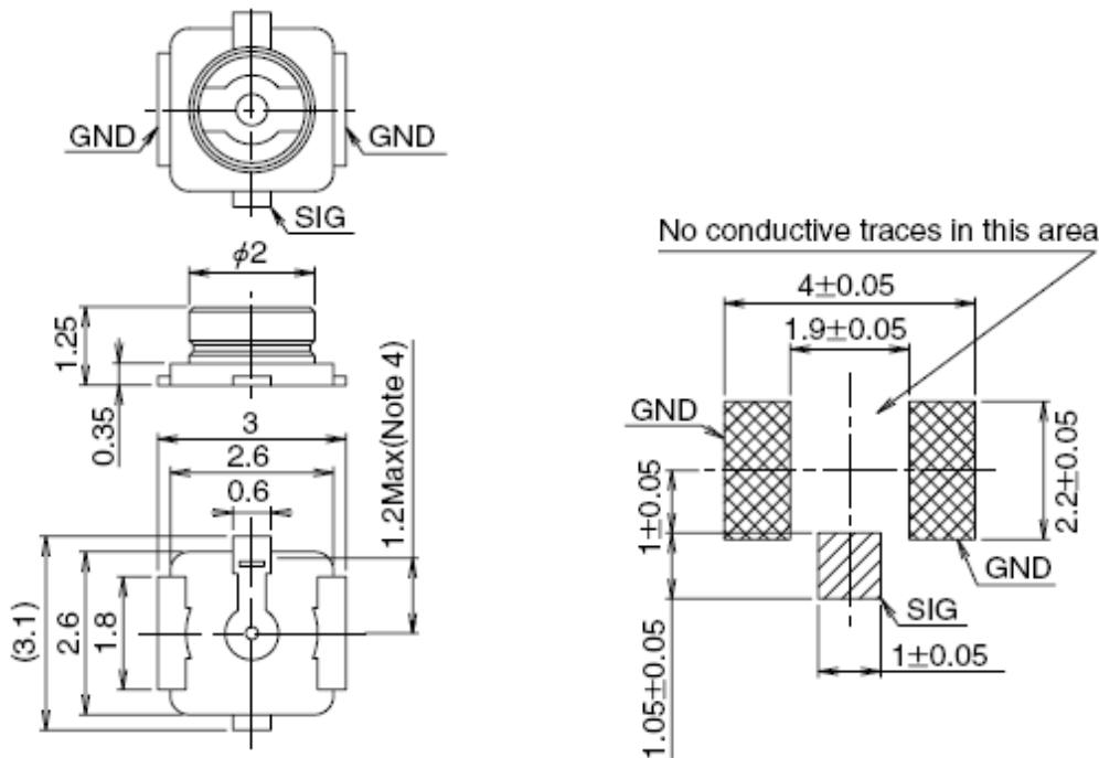
Figure 42: Dimensions of the U.FL-R-SMT Connector (Unit: mm)
