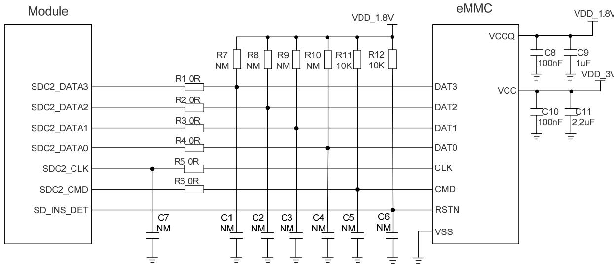
Figure 28: Reference Circuit Design for eMMC Application
