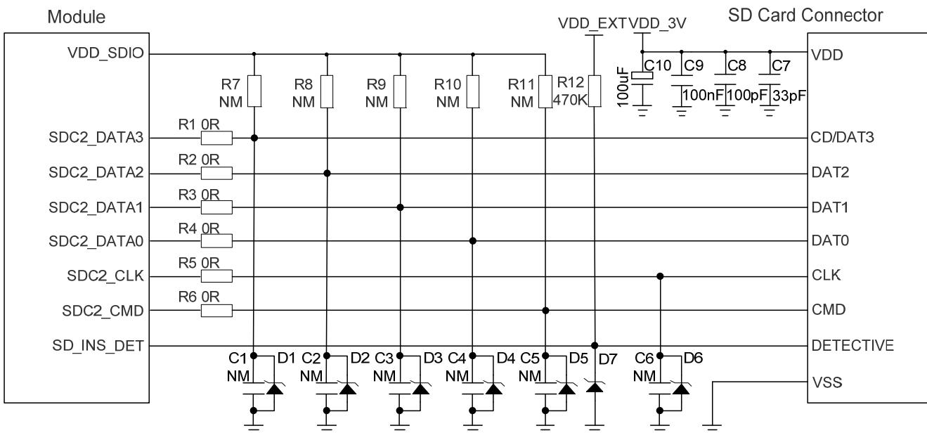
Figure 27: Reference Circuit Design for SD Card Application
