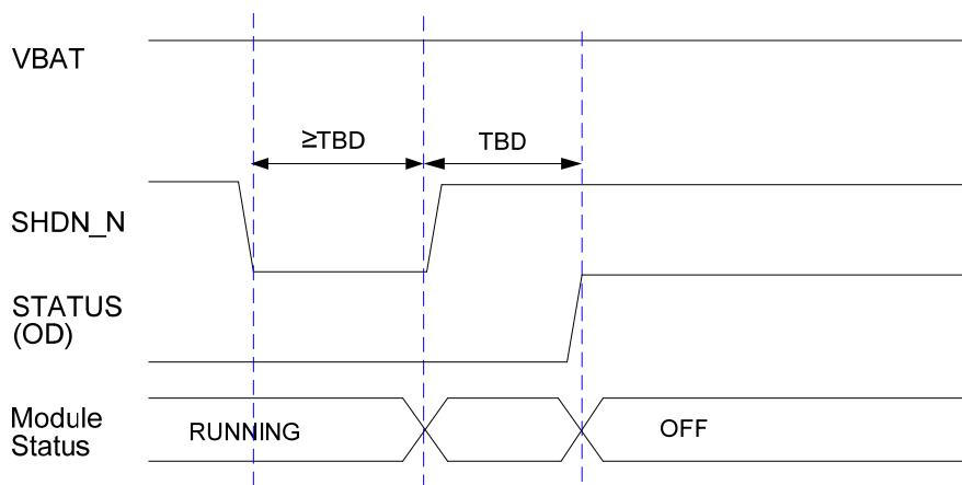
Figure 15: Timing of Turning off Module via SHDN\_N
