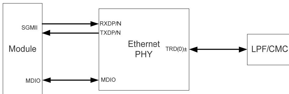
Figure 30: Simplified Block Diagram for Ethernet Application
