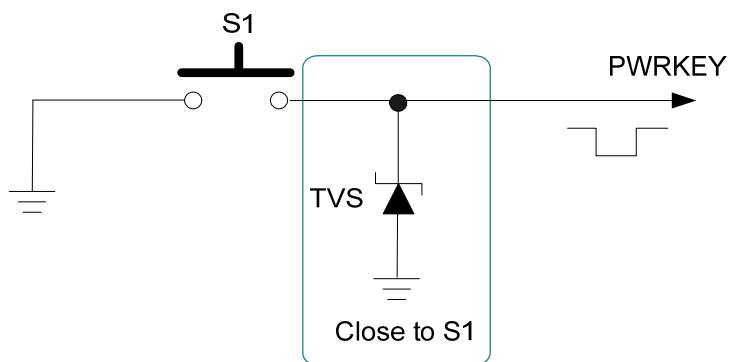
Figure 11: Turn on the Module Using Keystroke
