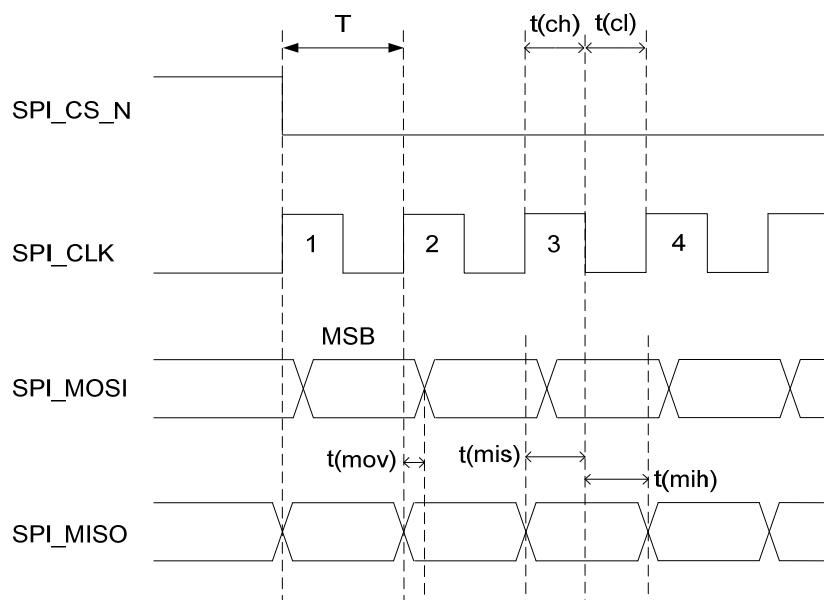
Figure 29: SPI Timing
