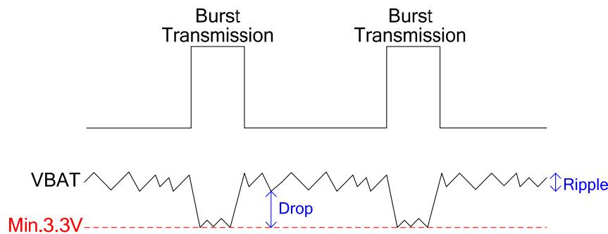
**Figure 7: Power Supply Limits during Burst Transmission**
