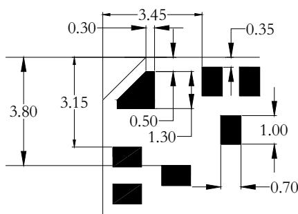
Figure 49: Recommended Footprint (Top View)
