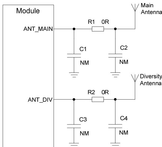
Figure 36: Reference Circuit of RF Antenna Interfaces
