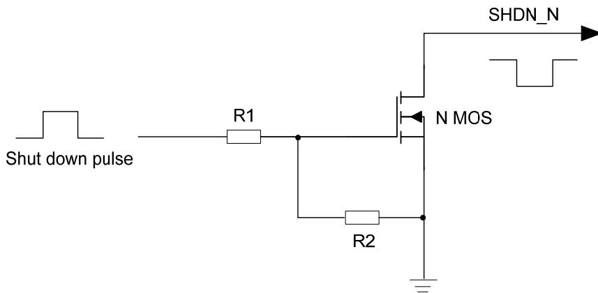
Figure 14: Shut Down the Module Using Driving Circuit
