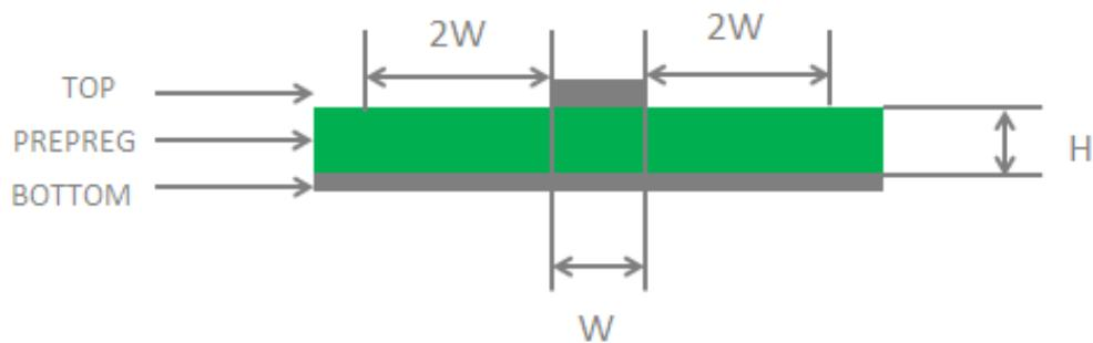
Figure 37: Microstrip Design on a 2-layer PCB
