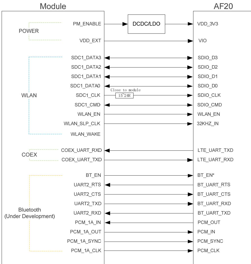
Figure 32: Reference Circuit for Connection with AF20 Module
