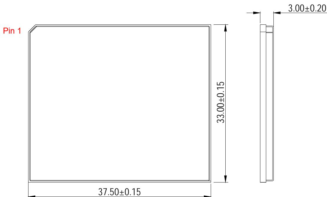
Figure 47: Module Top and Side Dimensions
