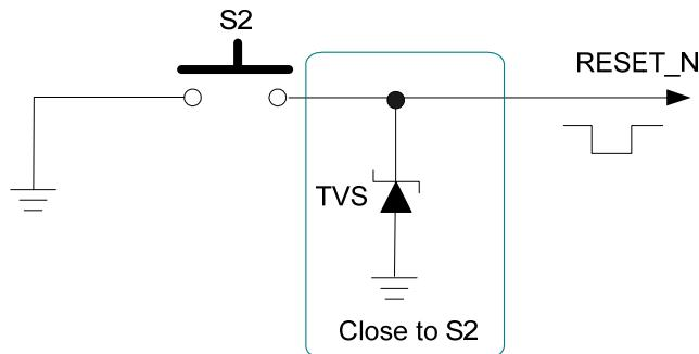
**Figure 17: Reference Circuit of RESET\_N by Using Button**
