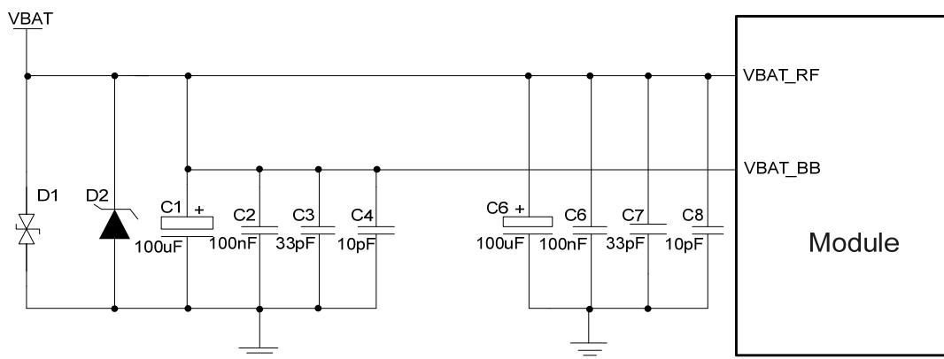
**Figure 8: Star Structure of the Power Supply**
