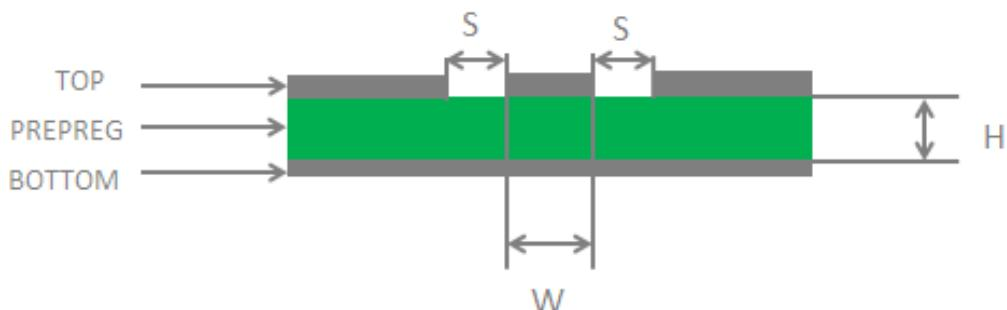
Figure 38: Coplanar Waveguide Design on a 2-layer PCB
