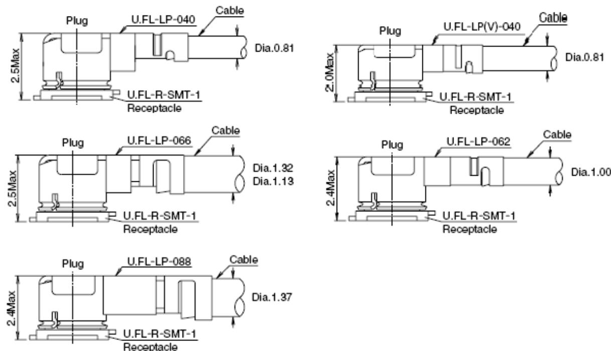
**Figure 44: Space Factor of Mated Connector (Unit: mm)**
