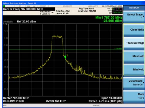
LTE Band 13 16QAM 10MHz CH-High, 1 RB
