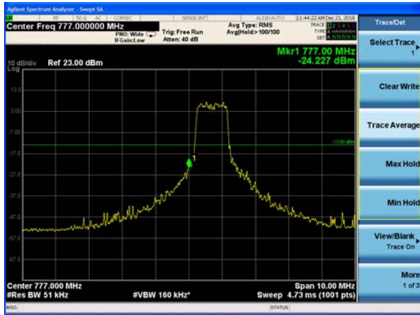
LTE Band 13 16QAM 10MHz CH-Low, 1 RB
