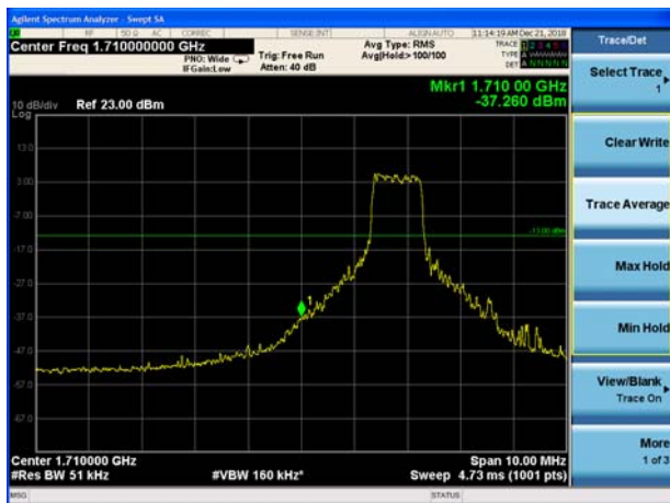
LTE Band 4 16QAM 20MHz CH-Low, 100%RB
