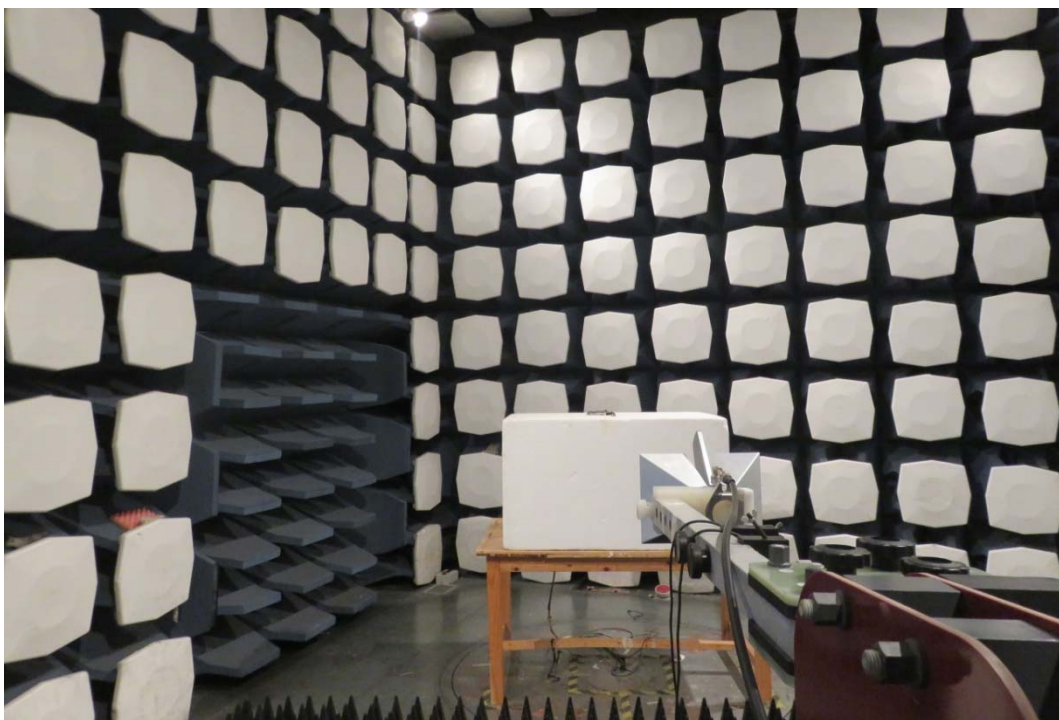
Picture 2 Radiated Spurious Emissions Test setup
