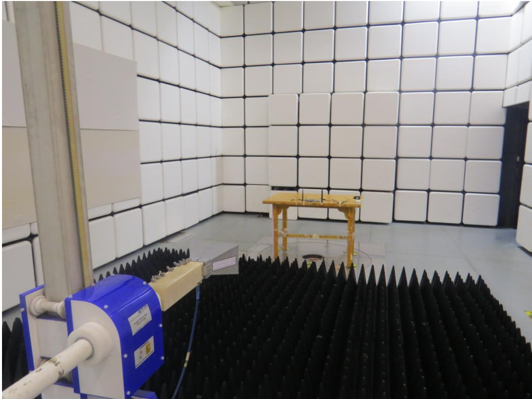
Picture 2: Radiated Spurious Emissions Test setup
