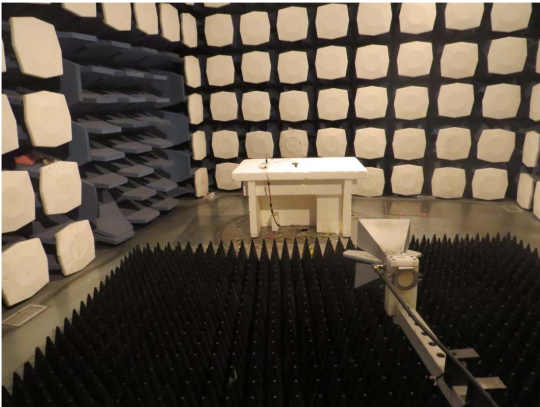
Picture 2: Radiated Spurious Emissions Test setup
