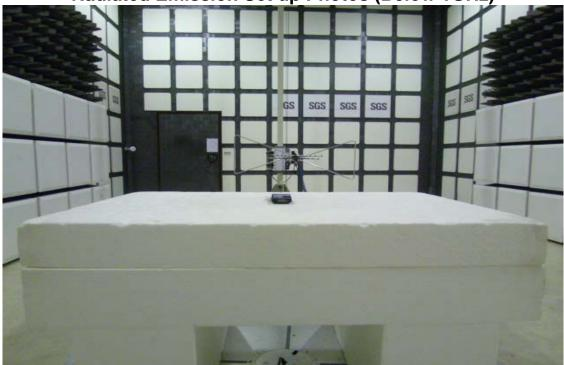
Radiated Emission Set up Photos (Above 1GHz)
