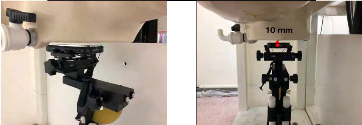
Fig.7 EUT Front side to flat phantom
