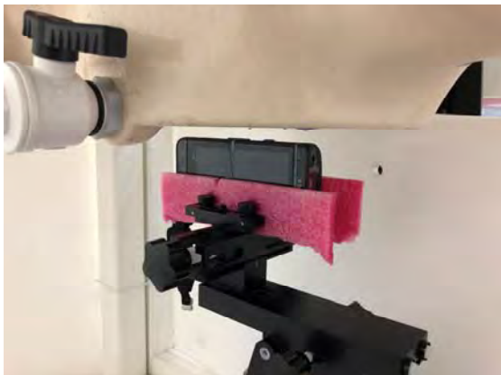
Fig.14 EUT Left side to flat phantom
