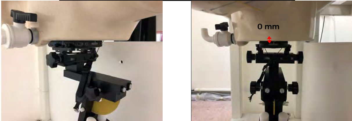
Fig.15 EUT Front side to flat phantom
