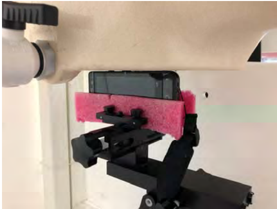
Fig.18 EUT Right side to flat phantom
