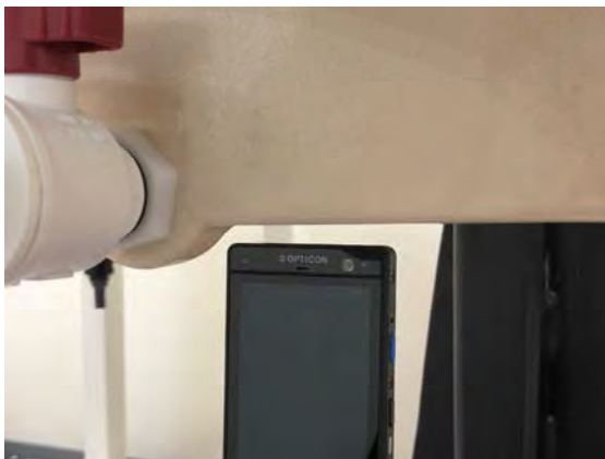
Fig.11 EUT Top side to flat phantom
