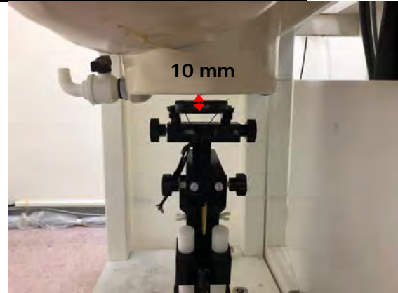
Fig.9 EUT Front side to flat phantom
