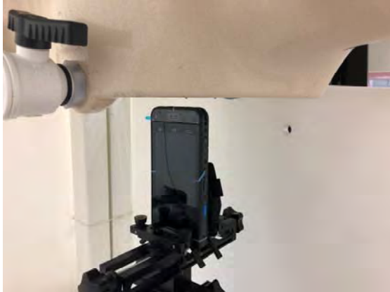
Fig.12 EUT Bottom side to flat phantom
