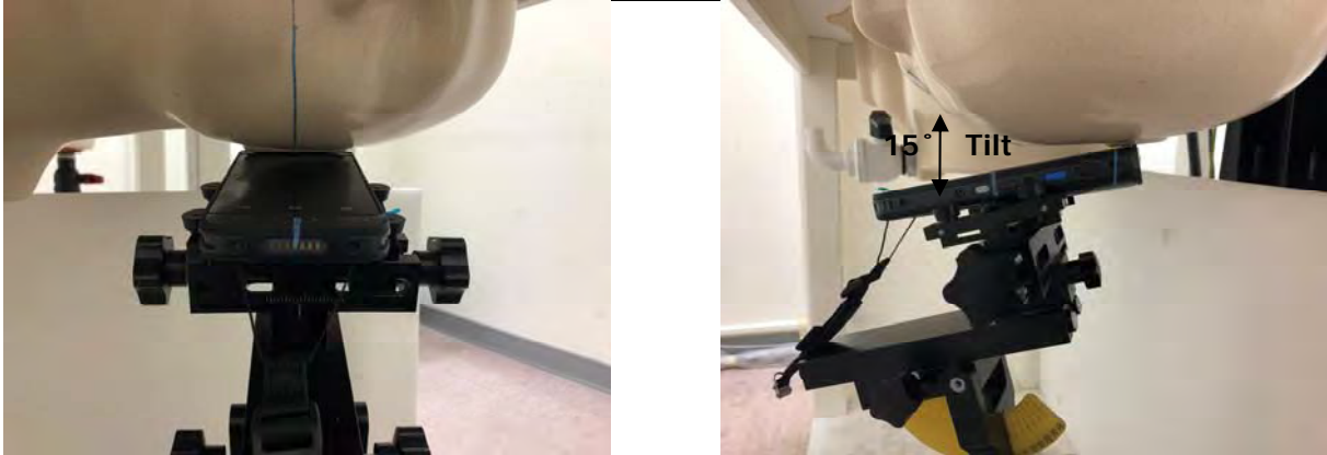
Fig.6 Left Head Section / Ear-Tilt Position(15°)
