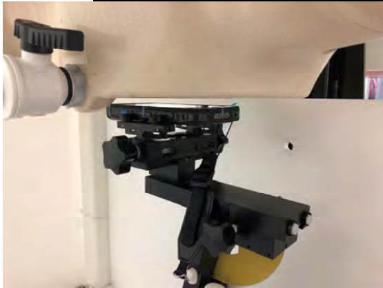
Fig.9 EUT Front side to flat phantom
