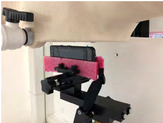
Fig.13 EUT Right side to flat phantom
