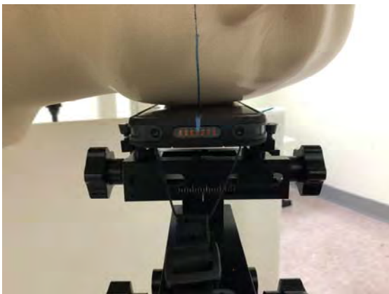
Fig.5 Left Head Section / Cheek-Touch Position
