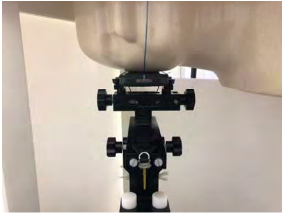
Fig.3 Right Head Section / Cheek-Touch Position
