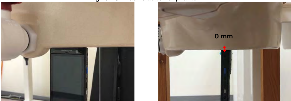
Fig.17 EUT Top side to flat phantom
