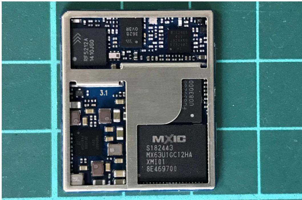
No shielding Front Side
