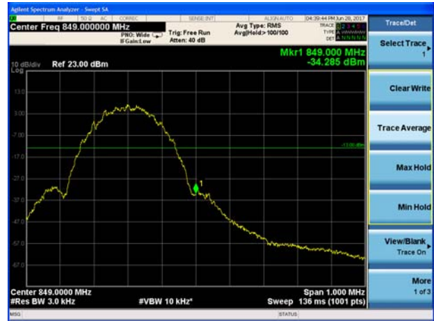
LTE Band 5 QPSK 1.4MHz CH-High 1RB
