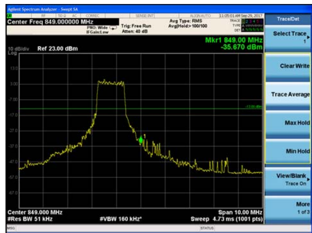
LTE Band 5 16QAM 1.4MHz CH-High 1RB
