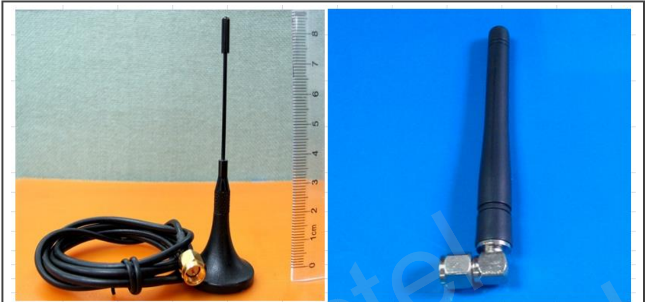
Figure 15: Example of Practical Monopole Antennas
