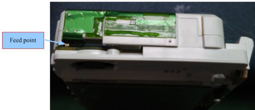
Figure 6: Example of FPC Monopole Antenna
