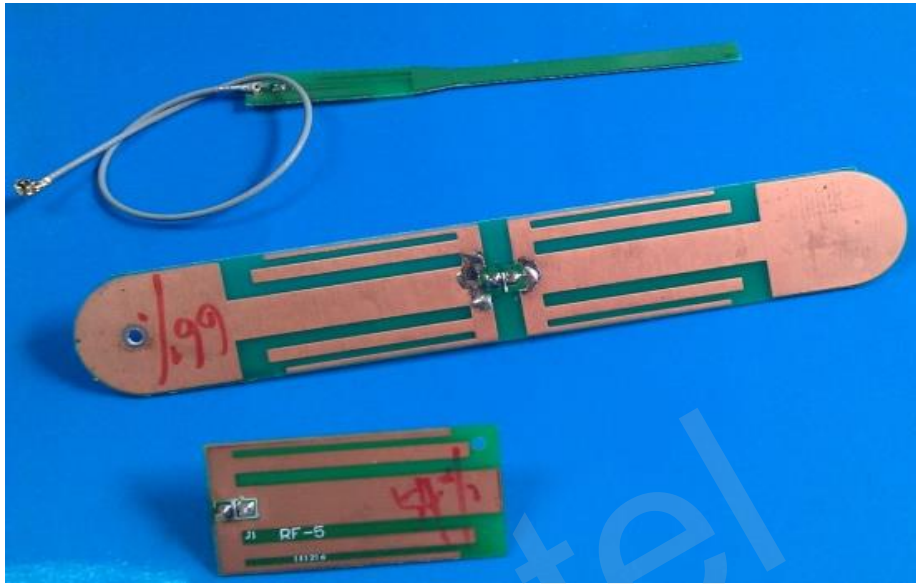
Figure 10: Example of PCB Antenna
