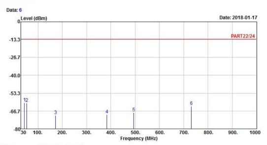
Site : 966 Chamber 5 Condition: PART22/24 VERTICAL Remak : EDGE 1900 Link\_L-CH
