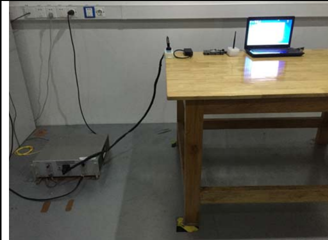
Conducted Emissions Test Setup Front View
