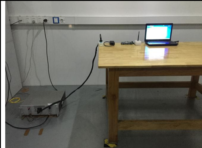
Conducted Emissions Test Setup Front View
