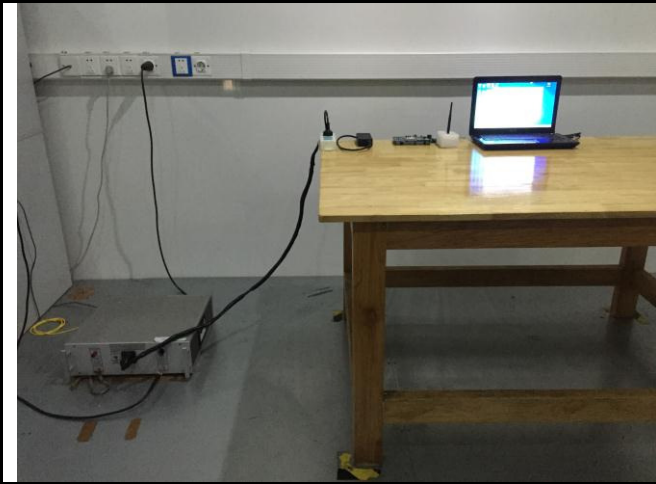
Conducted Emissions Test Setup Front View
