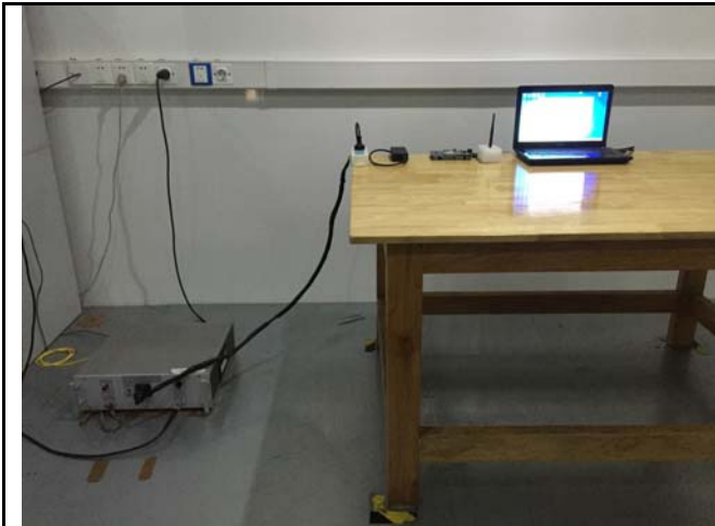
Conducted Emissions Test Setup Front View
