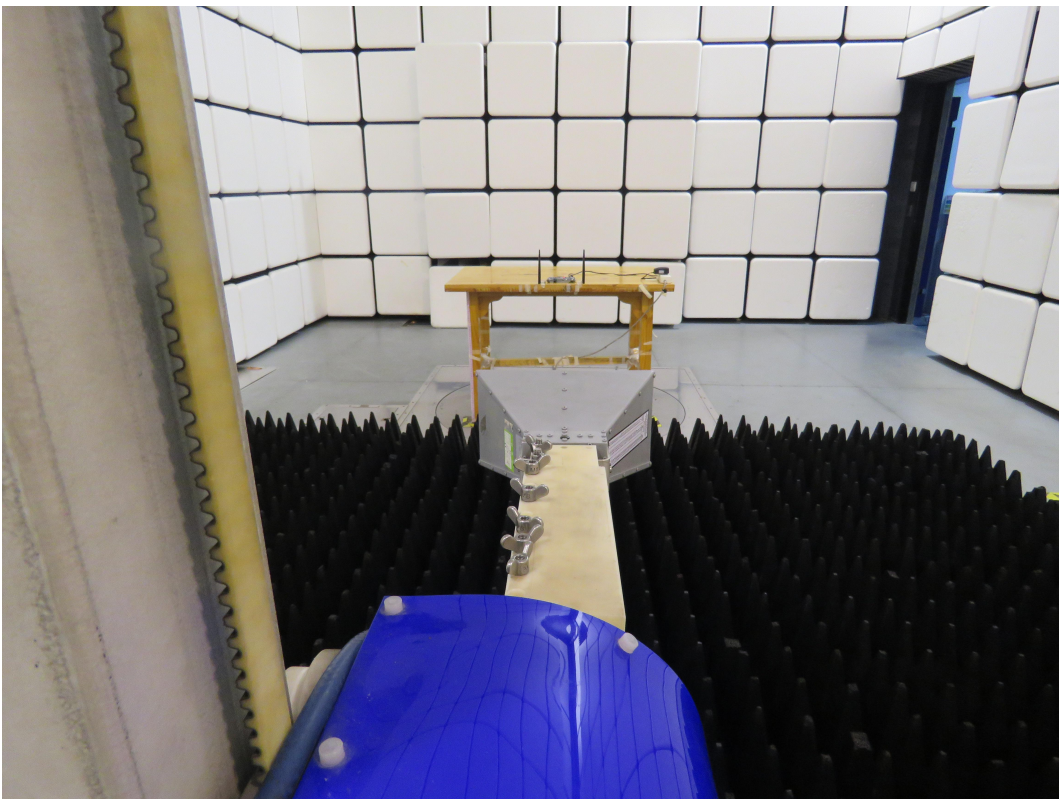
Picture 2: Radiated Spurious Emissions Test setup
