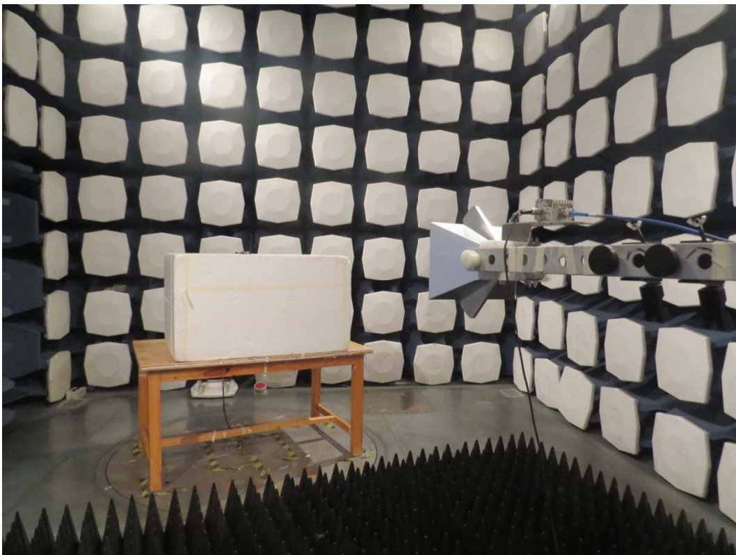
Picture 2 Radiated Spurious Emissions Test setup
