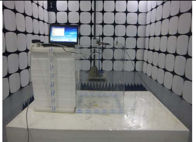
Radiated Spurious Emissions Test Setup Above 1GHz
