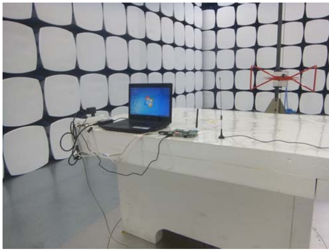
Radiated Spurious Emissions Test Setup Below 1GHz
