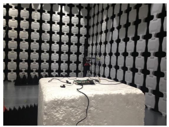
Description: Substitution Antenna for EIRP Test
