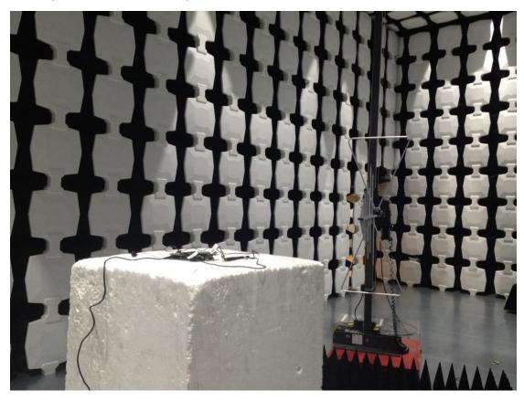
Description: Substitution Antenna for ERP Test
