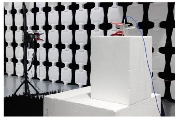
**Test Photograph**Description: Conducted Emission Test Setup
