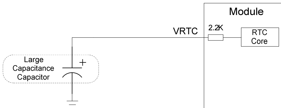
Figure 17: RTC Supplied from a Capacitor
